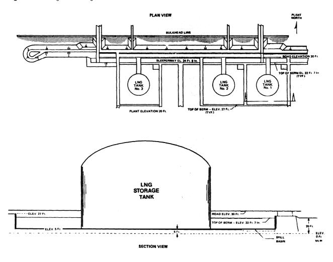
Figure 21. Storage and Diking at Onshore LNG Plant
