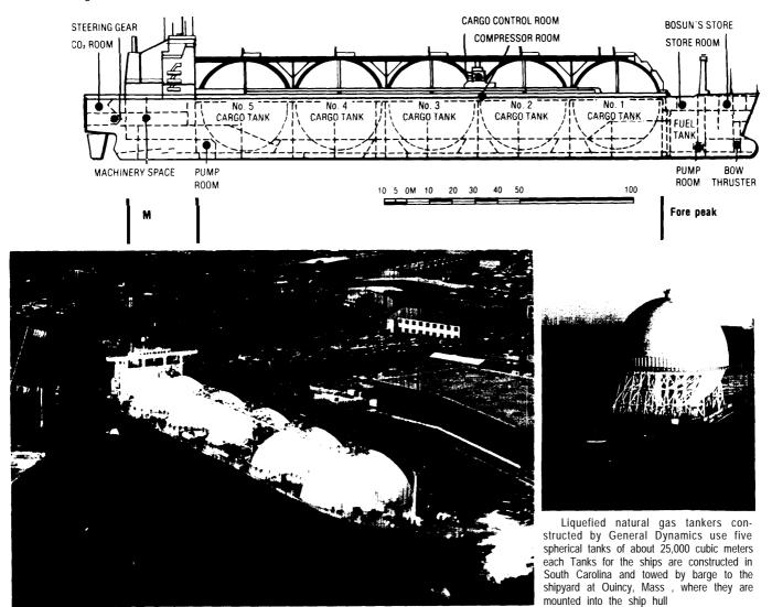
Figure 12. Inboard Profile of LNG Tanker
