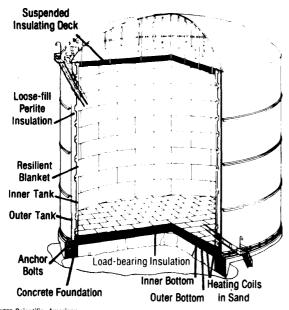
Figure 18. AbovegroundLNG Storage Tank
