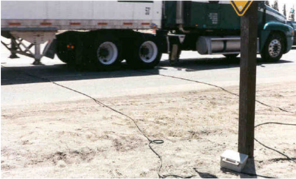
Figure 7: Photo of Pressure Tube Speed Detectors at Eisenhower Tunnel
