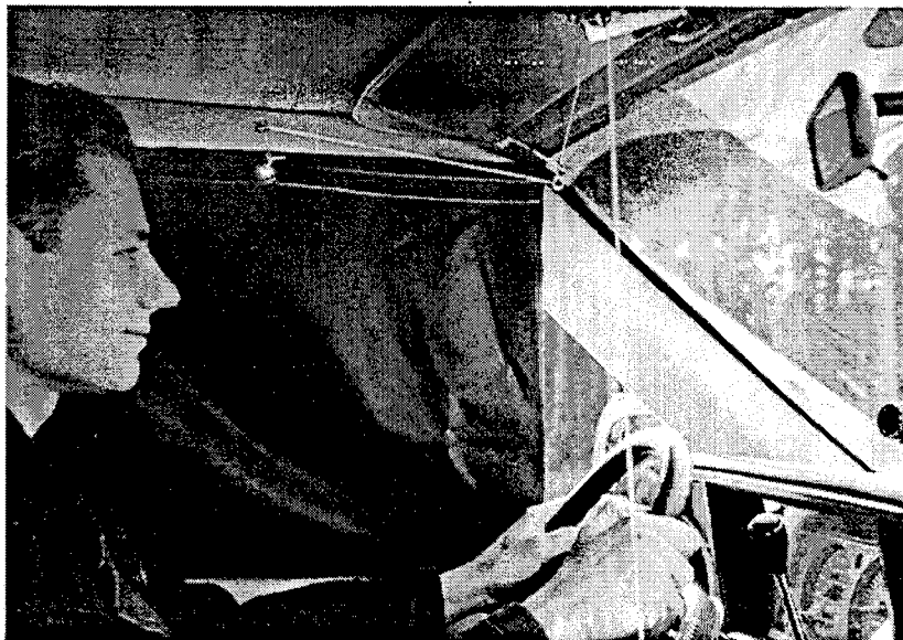
Figure 25 Curtain closed to block the field of view through the left window and in the driver's side mirror.
