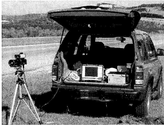
Figure C-5. Typical TMS Setup.
