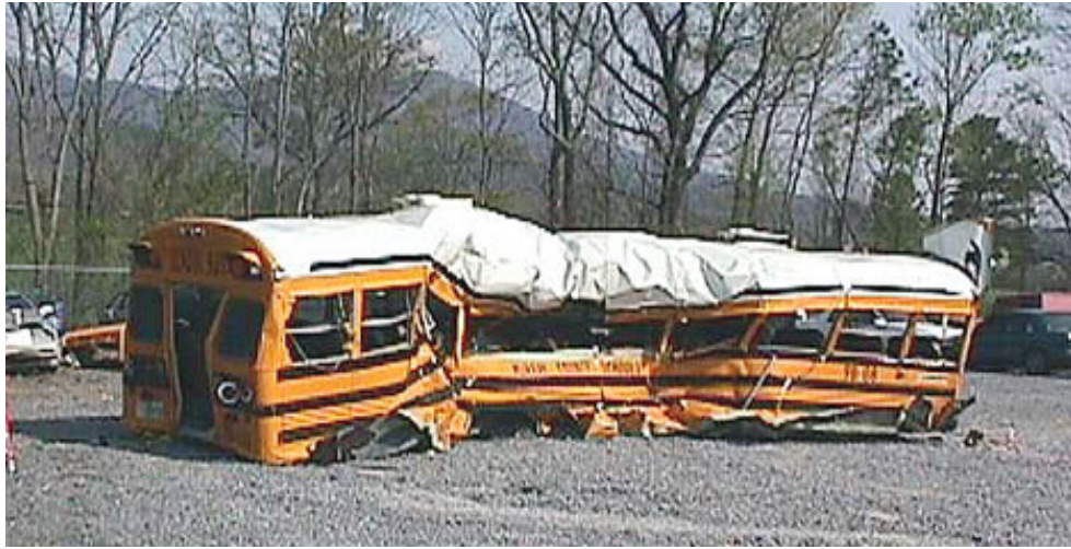
Figure 9. School bus exterior body damage.
