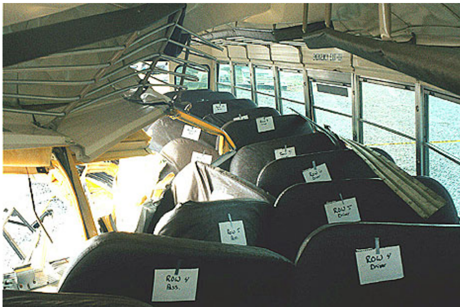
Figure 10. School bus interior body damage.
