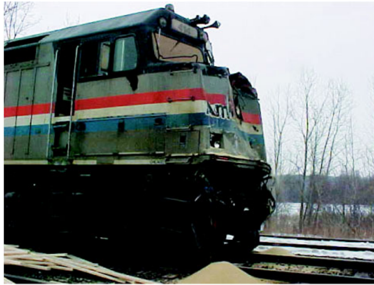
Figure 6. Damaged lead locomotive of Amtrak train 286.
