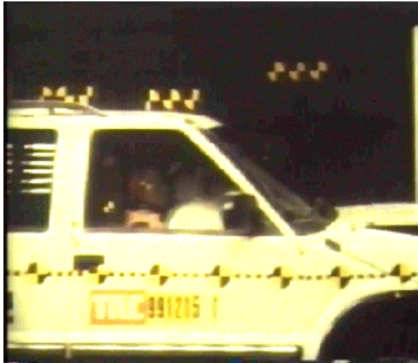
Figure 5: MY 1999 Chevrolet Blazer (NHTSA Test # V3222); Initial passenger air bag deployment toward the chest
