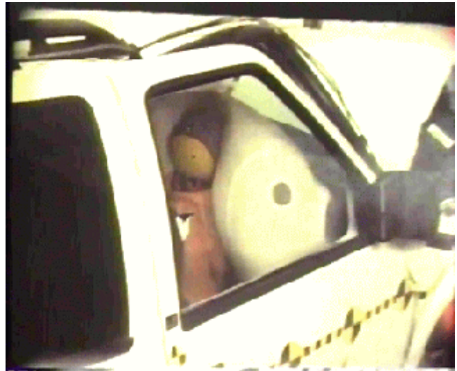
Figure 6: Dummy head-to-windshield contact through the passenger air bag.
