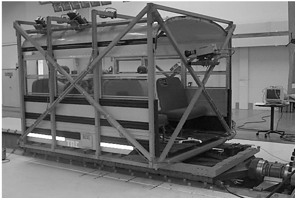
Figure 11. First Sled Buck used in Simulating Frontal Crashes
