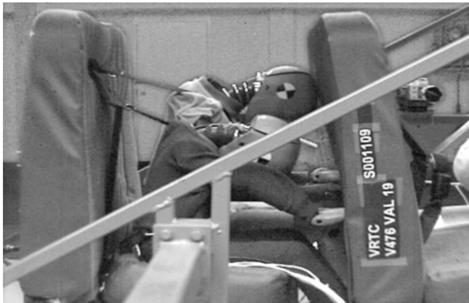
Figure 21. Lap/Shoulder Belt Test at Maximum Neck Flexion
