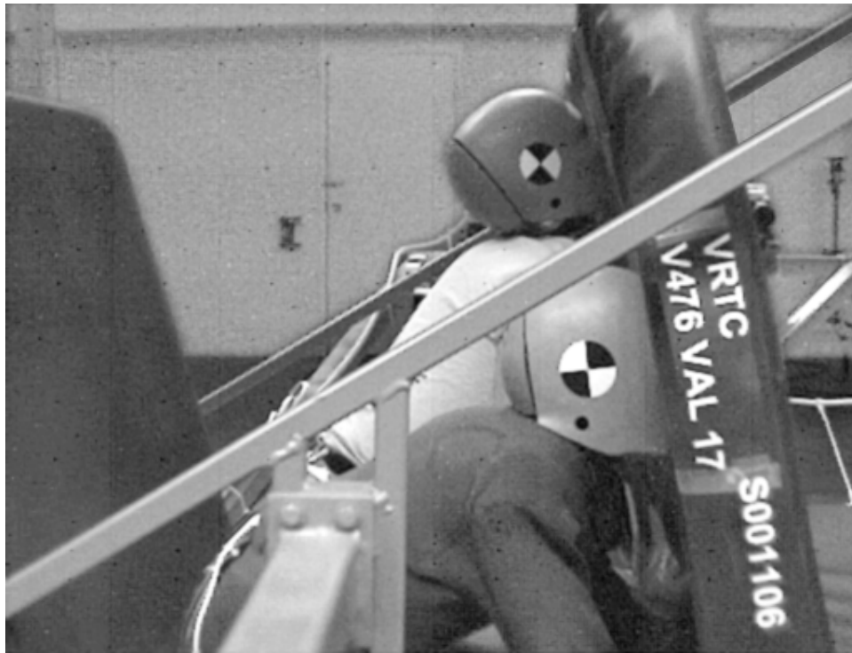
Figure 20. Lap Belt Test at Maximum Neck Extension, 150 msec
