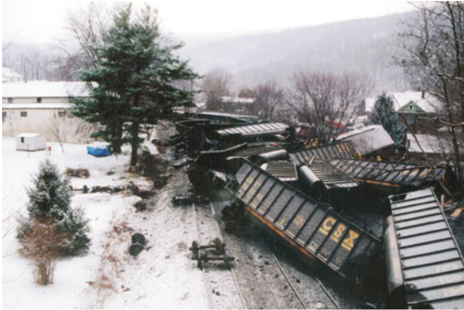
Figure 3. Pileup of derailed coal cars.
