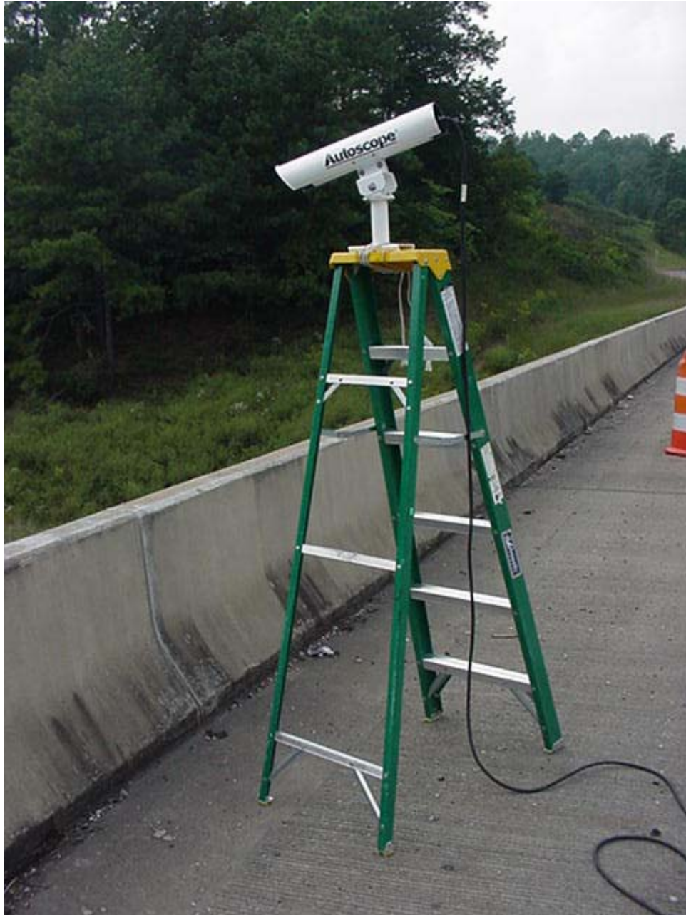
Figure 4-3. Placement of Machine Vision Processor Camera on An Overpass.
