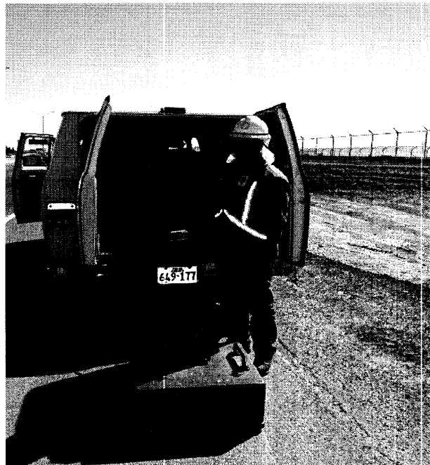
Figure 3. Data Collection with a 200 MHz Ground-Coupled System.
