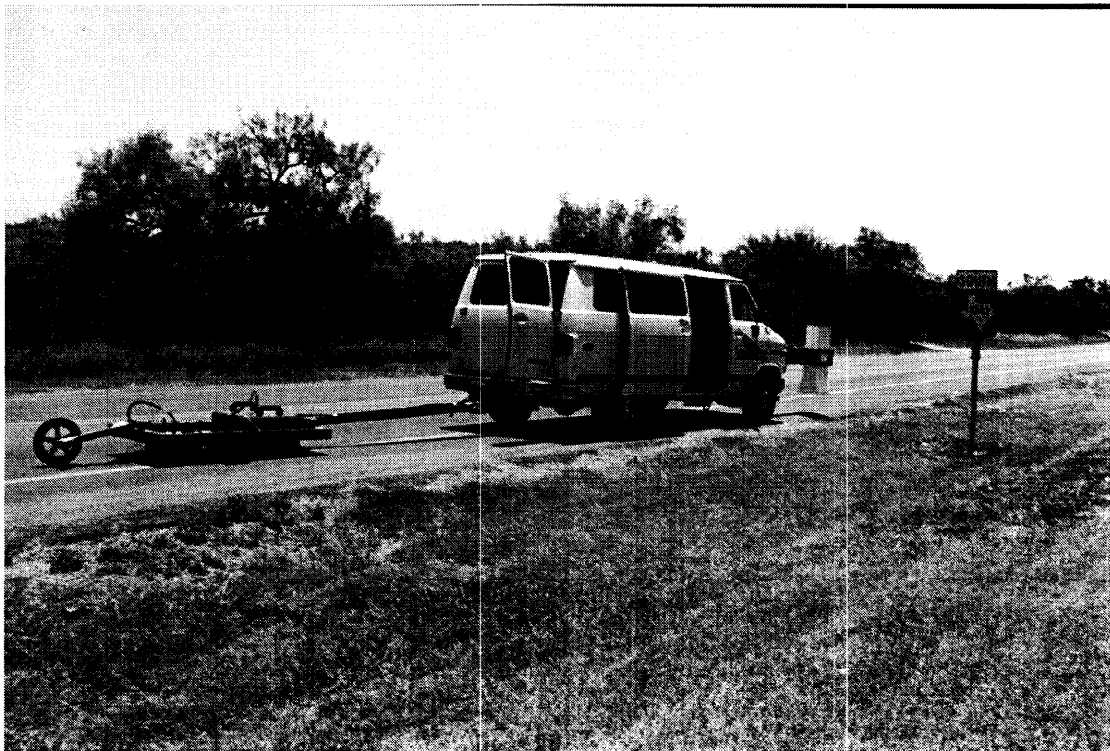
Figure 4. Simultaneously Collecting Air-Launched and Ground-Coupled GPR Data.
