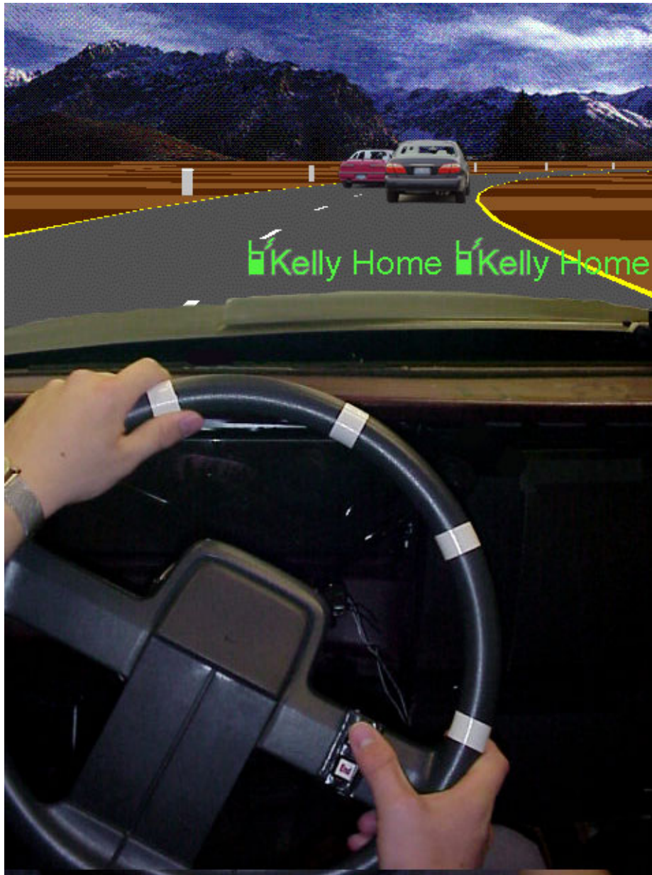
Figure 6. Cell phone buttons on the steering wheel ( HUD images enlarged by 50% ).
