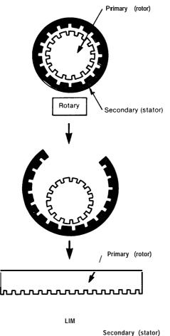
Figure 10.—The Principle of Linear Motors
