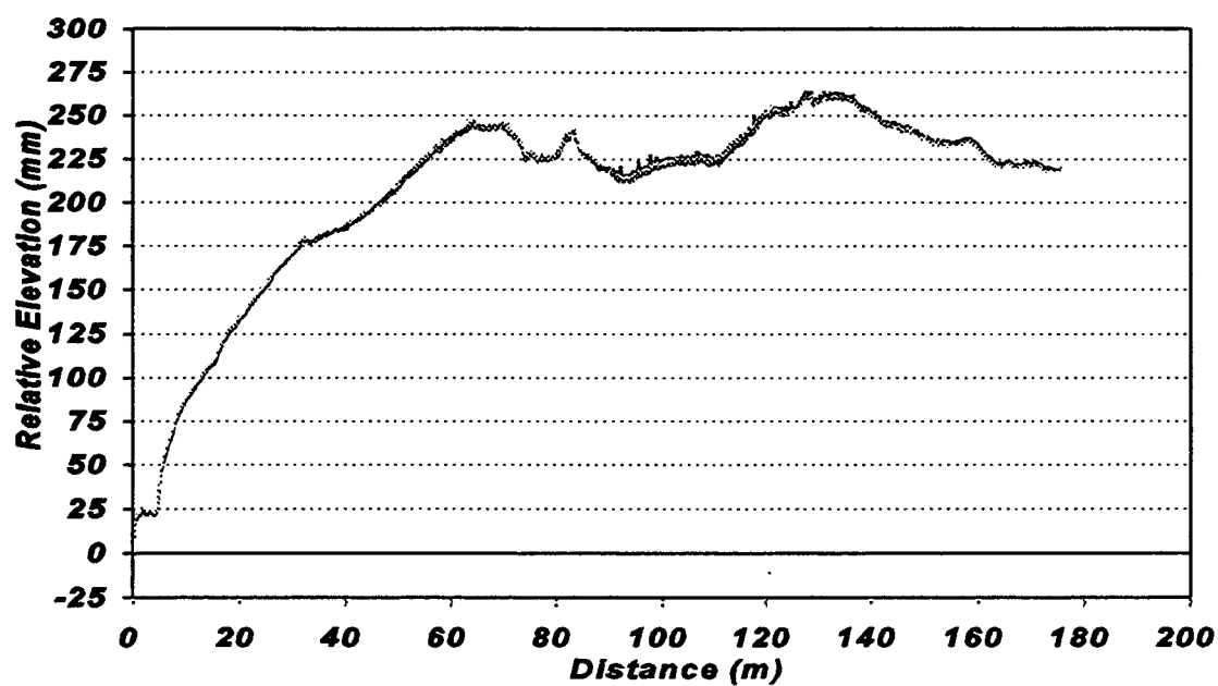
Figure A1. Original Profiles from Rod & Level on Annex 1 Site.
