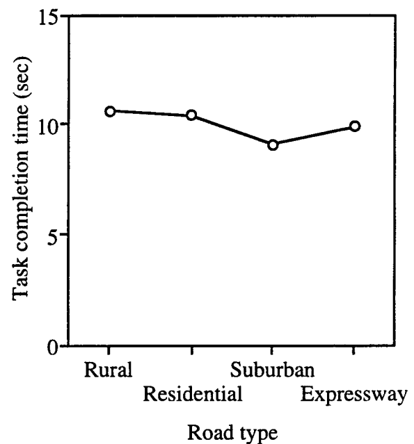
Figure 2.3.15. Effect of context on task completion time (on the road)
