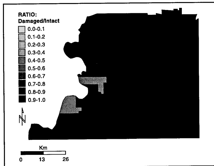
■ Figure 3.7 Ratio of the Average Power Output under the Damaged Condition to the Intact Condition for Service Areas ( M = 7.0 )
