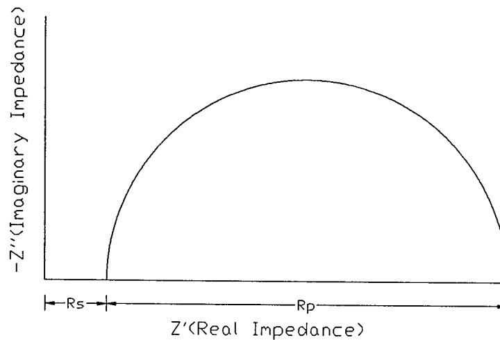
Figure 3.4 Nyquist Plot for Electrical Circuit Shown in Figure 3.2.
