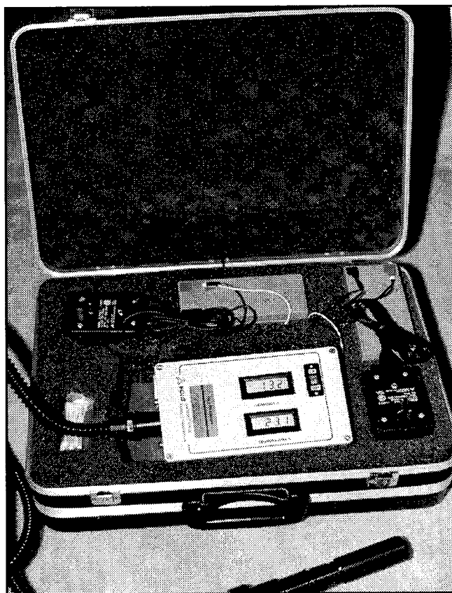
Figure 3.22 View of the Dew Point Indicator.
