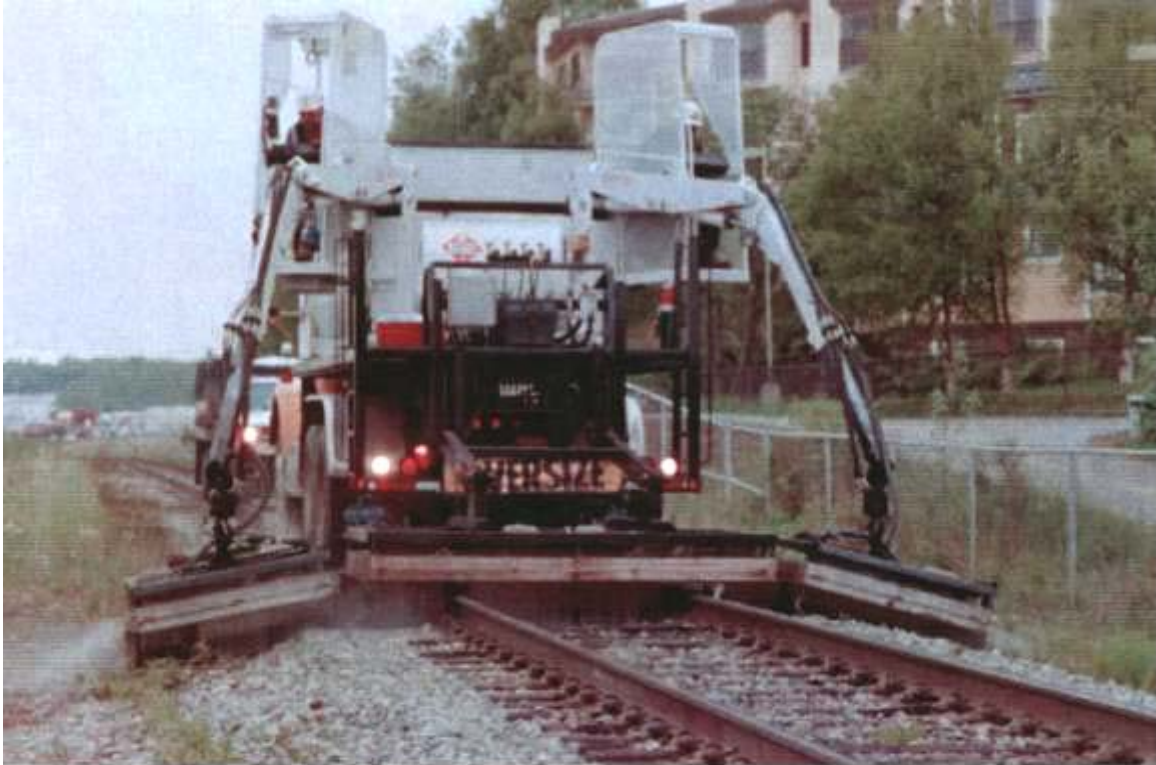
Figure 4: Hy-Rail infra-red platform tested in Alaska.
