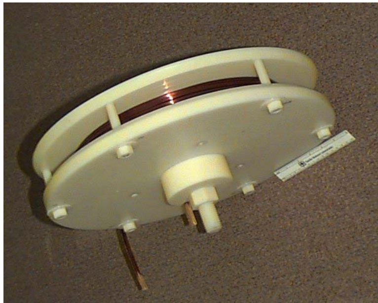
Figure 17. Test coil in dielectric housing to measure winding resistance increase due to eddy currents. Outer diameter of housing is 45.7 cm.
