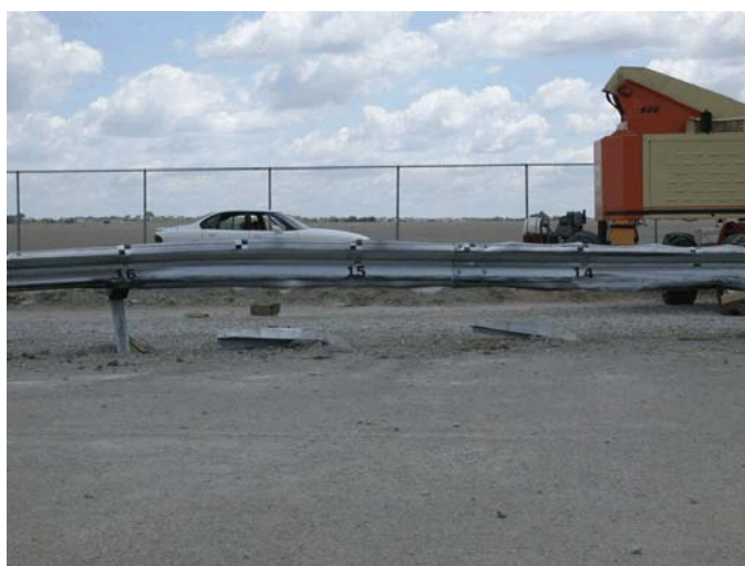
Figure 95. System Damage, Test NPG-4
