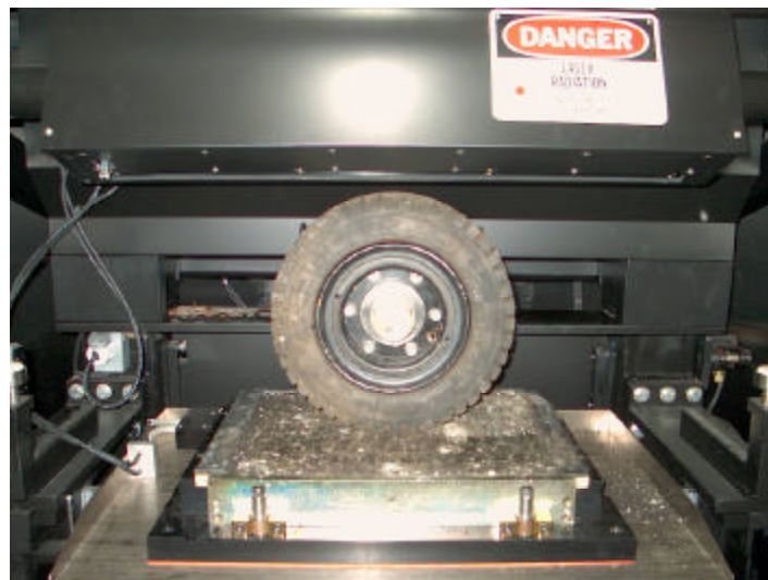
Figure 5.19 Typical Rut Test Using the NCSU WTD
