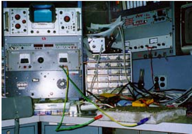
Figure 3-7 Small conductive concrete slab heating test
