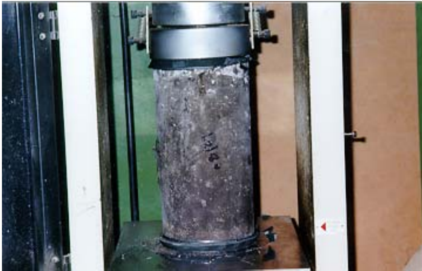
Figure 4-4 Typical failure mode of concrete in compression
