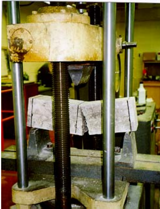
Figure 4-8 Flexural strength – test setup
