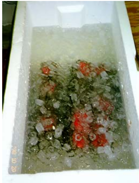
Figure 4-11 Freeze and thaw specimens during taking measurements
