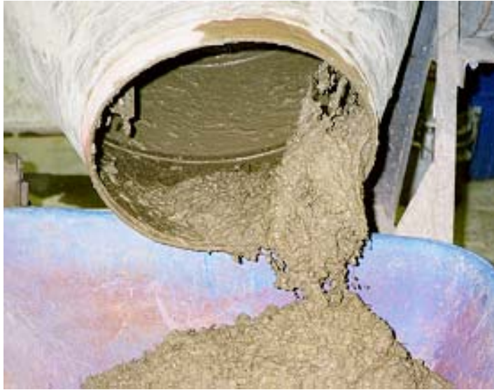
Figure 3-4 Typical conductive concrete mix
