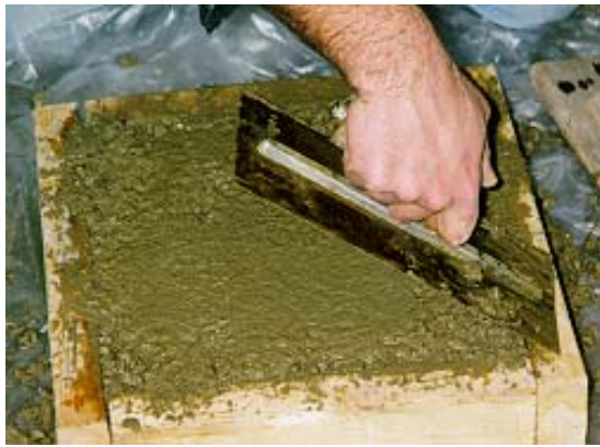
Figure 3-5 Surface finishability of conductive concrete
