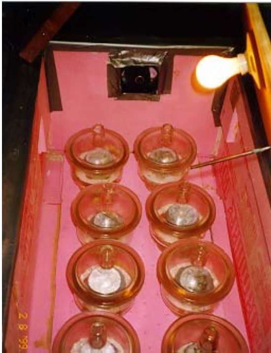
Figure 4-19 Specimens inside moisture-free desiccators
