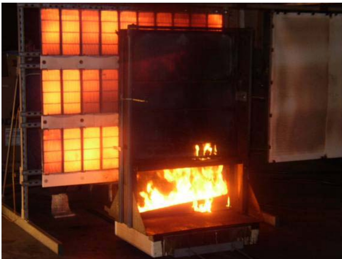
Figure 8. Air Ducts – ICAL Test in Progress.
