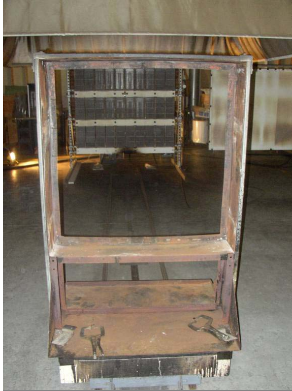
Figure 6. Close-up of Test Frame and Drip Pan for ICAL Apparatus.
