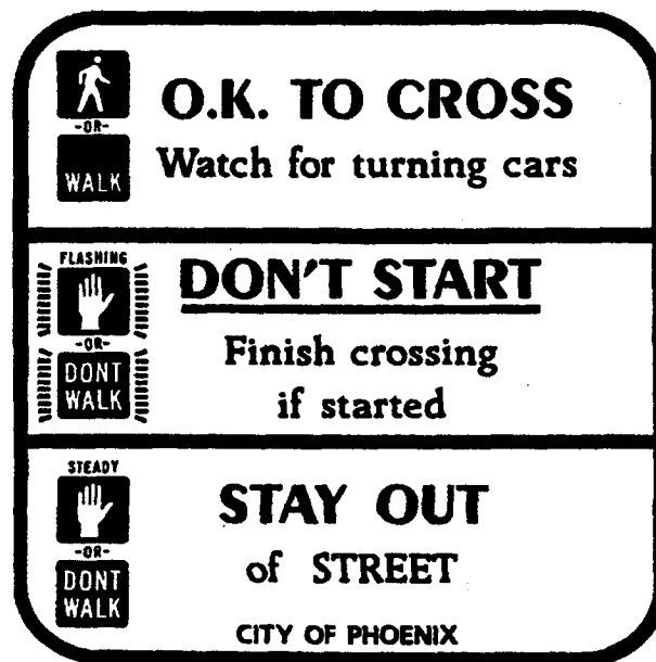
Figure 3. Phoenix pedestrian signal explanation sign.
