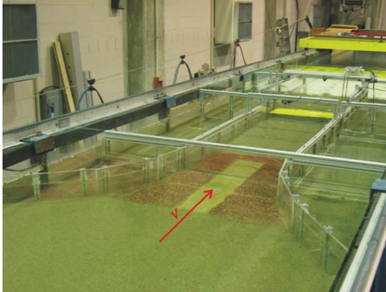
Figure 8. Photo. Approach section of the test flume.
