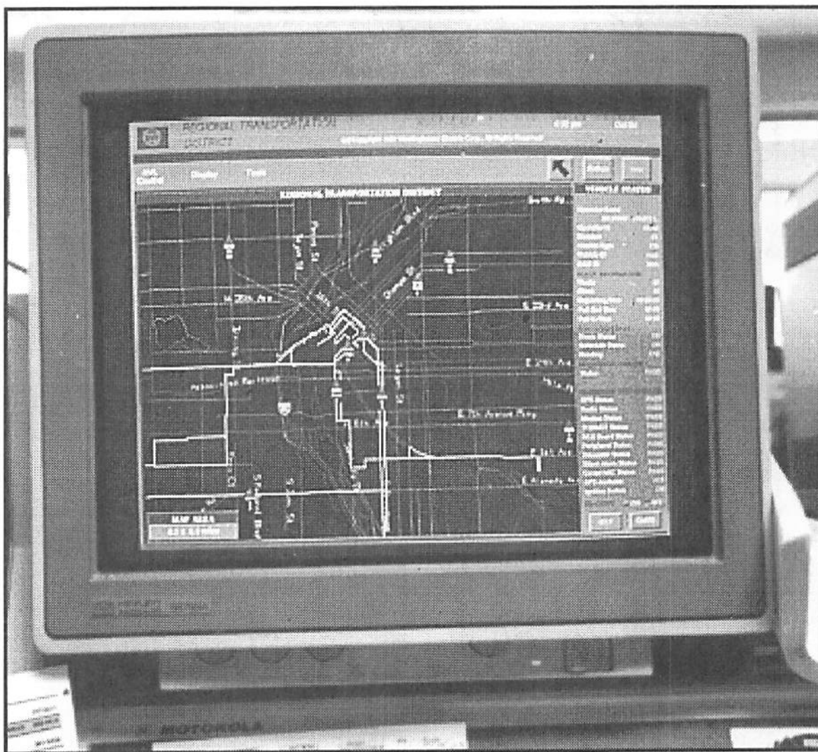
Figure 13. Automatic Vehicle Location Screen
