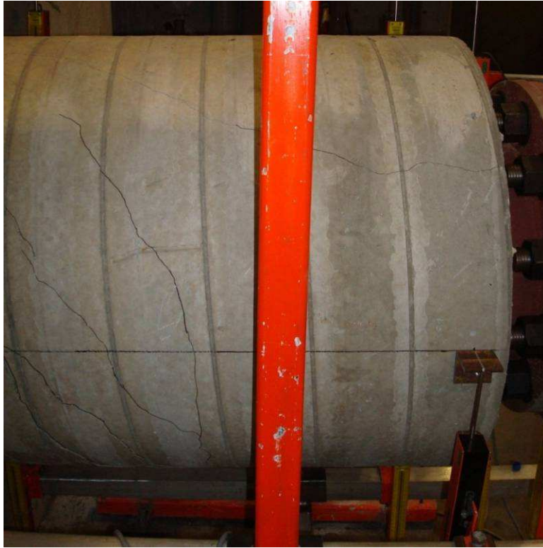
Figure 5-9. Torsional and flexural cracks forming
