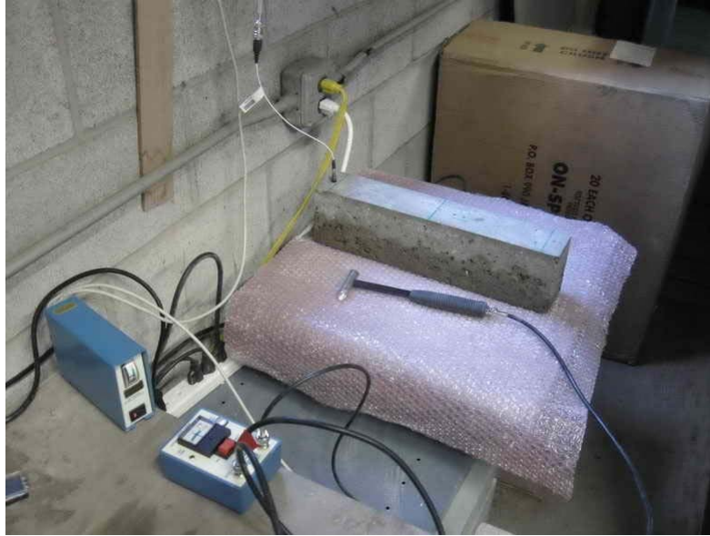
Figure 13. Dynamic Modulus of Elasticity (MOE) Test Setup
