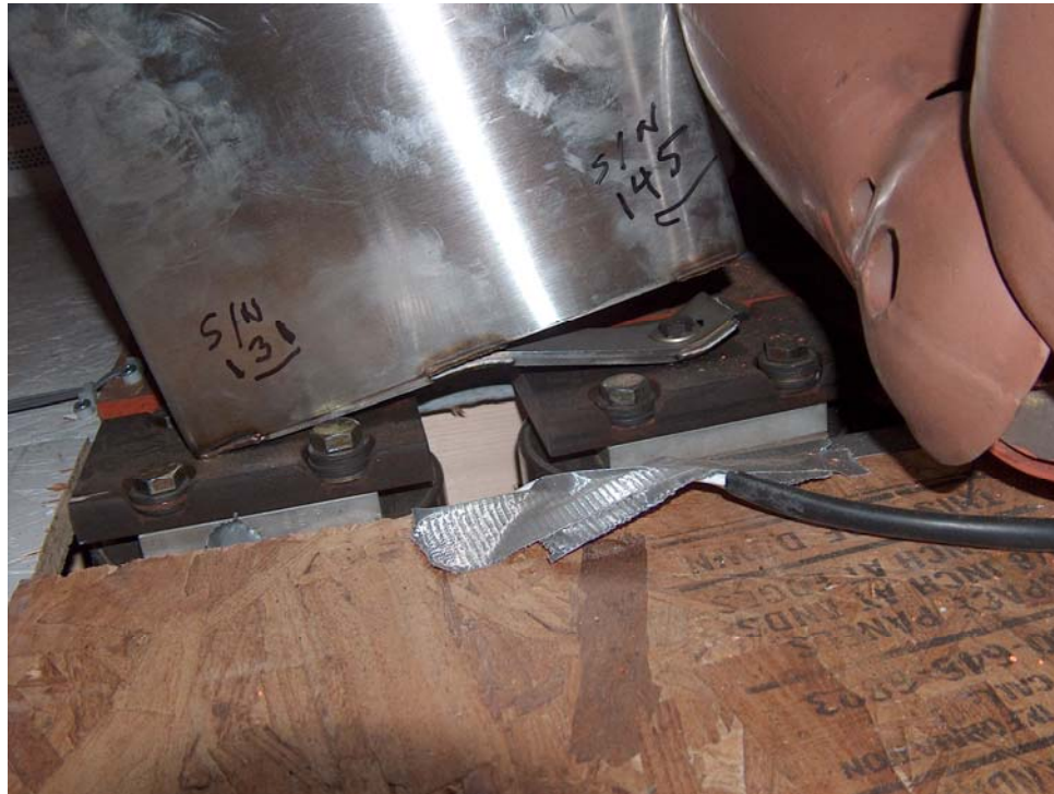
Figure 56. Weld Failure at Pedestal Base, which Caused the Seat to Rotate Forward and Allowed the ATDs to Fall into the Aisle in Experiment 2.2
