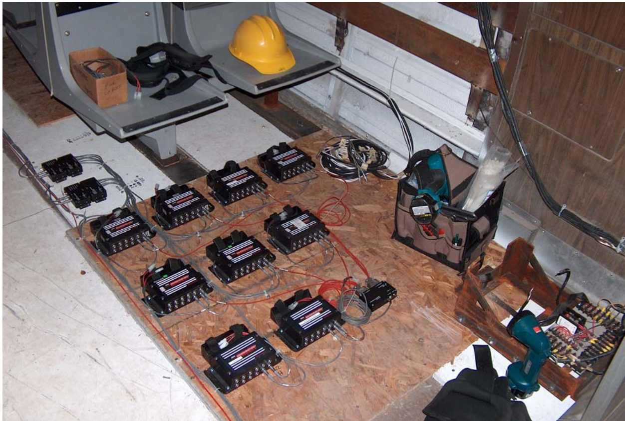
Figure 19. Nine Data Bricks Installed to Collect Data from 70 Channels Linked to Experiments 1.2 and 1.3
