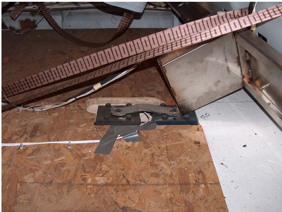
Figure 46. Weld Failure at the Pedestal Base, which Caused the Seat to Collapse in Experiment 1.1
