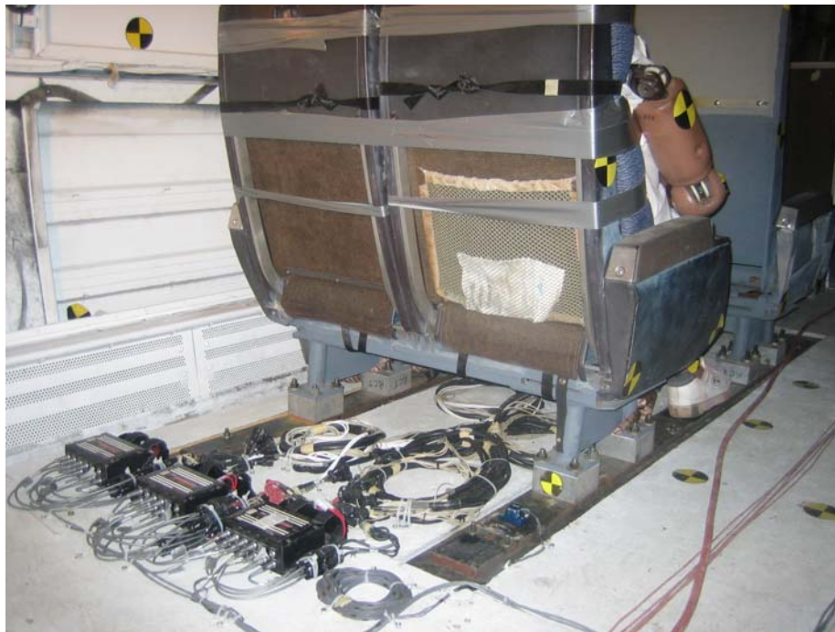
Figure 31. Three Data Bricks and One Accelerometer, Installed behind Experiment 2.1
