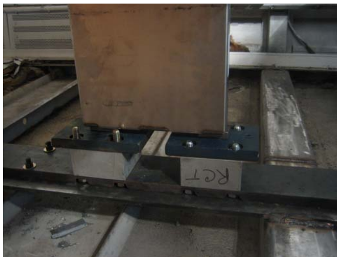
Figure 5. Floor-Attachment Spacer Blocks for Unoccupied Rebound Seat (left) and Load Cells for Occupied Front-Row Seat (right) in Experiment 1.1
