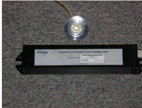
Figure 9-7. LED Emergency Light with Capacitive Energy Storage
