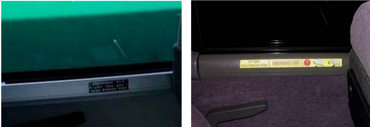
Figure 6-3. MCI Emergency Exit Window Release Bars
