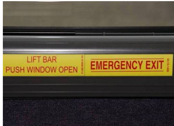
Figure 8-3. Motorcoach Emergency Exit Window Marking and Instructions (1)
