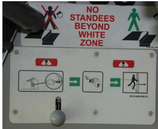
Figure 8-1. Motorcoach Front-Door Operation Instructional Signage Example – Interior
