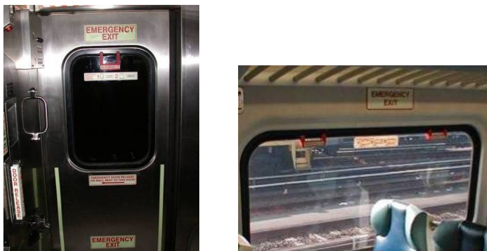
Figure 8-10. Passenger Rail Car – Photoluminescent Emergency Exit Signage
