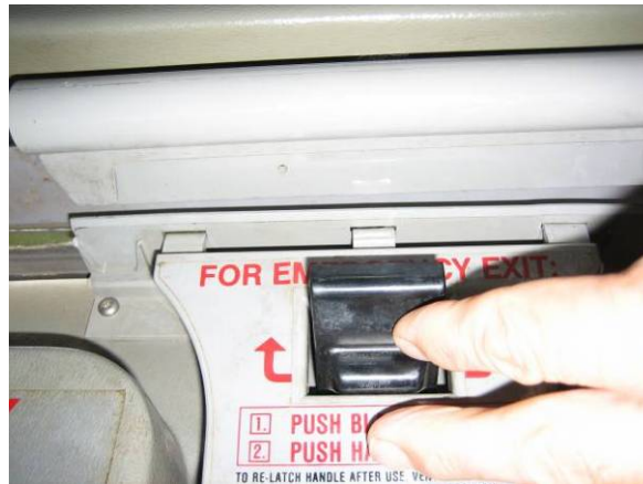
Figure 3-1. Fingertip Release – Emergency Roof Exit Hatch
