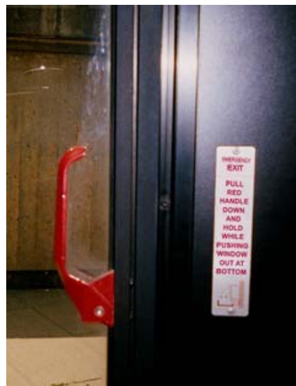
Figure 8-7. Transit Bus Door and Window Emergency Exit Signage – Interior
