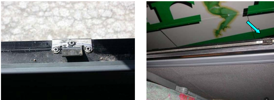
Figure 6-8. Van Hool Emergency Exit Window Sill-Mounted Release Components
