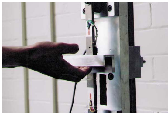
Figure 6-14. Test Apparatus for Measuring Finger-Tip Pulling Strength
