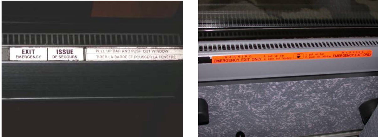
Figure 6-5. Prevost Sash-Mounted Emergency Exit Window Release Bars
