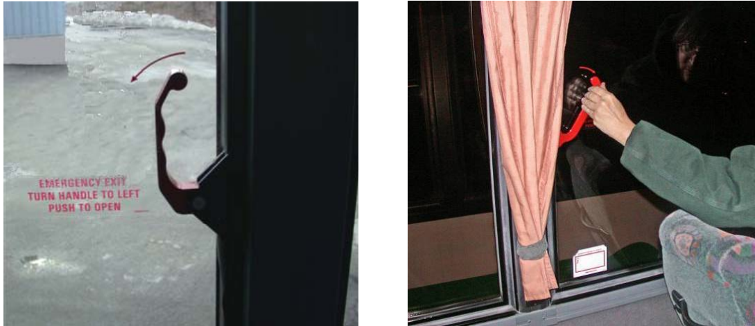
Figure 6-7. Van Hool Sash-Mounted Emergency Exit Window Release Mechanism
