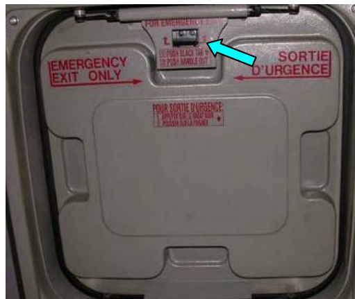
Figure 7-2. Prevost and Van Hool Emergency Roof Exit Hatch
