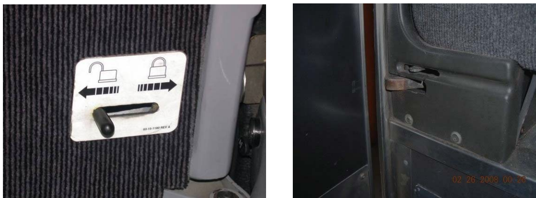
Figure 4-4. Motorcoach Interior Latches for Front Door
