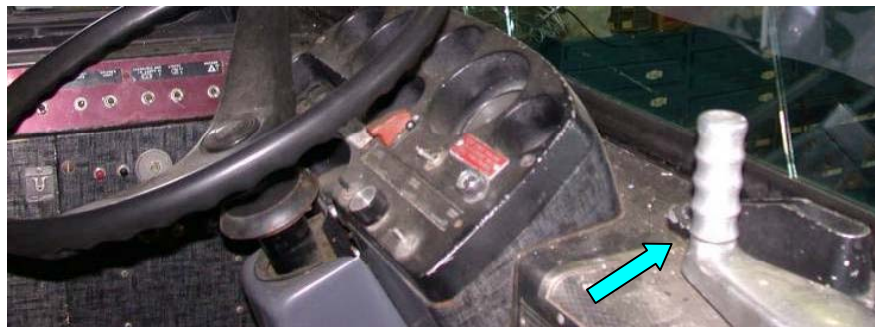
Figure 4-6. Hand-Crank Front Door Opener
