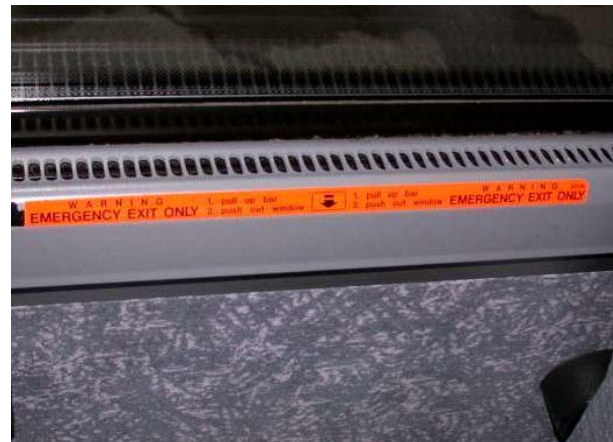
Figure 8-4. Motorcoach Emergency Exit Window Marking and Instructions (2)
