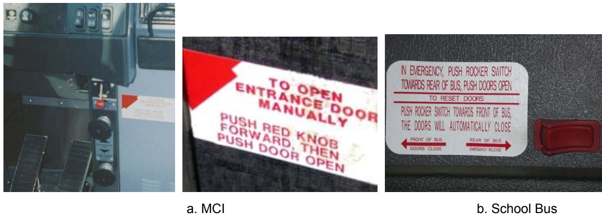
Figure 4-5. Door Pneumatic Actuator Pressure Release Knob and Instructions
