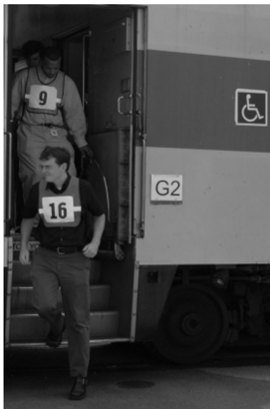
Figure 4-10. Volpe Center Commuter Rail Experiment to Measure Normal Egress Rate
