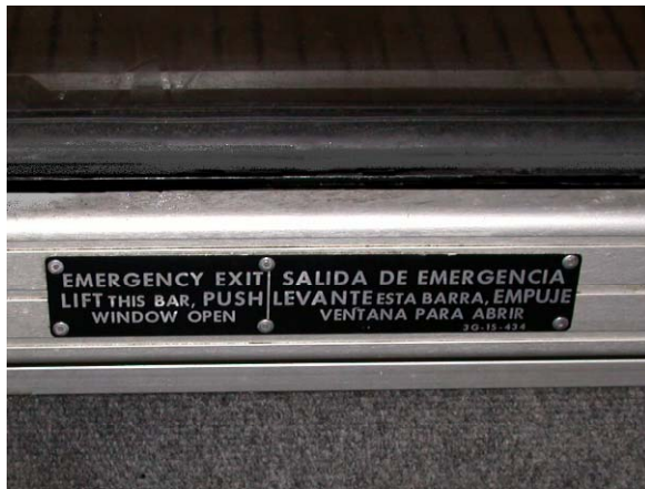
Figure 8-3. Motorcoach Emergency Exit Window Marking and Instructions (1)
