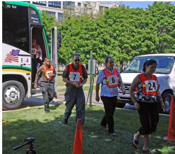
Figure 4-9. Volpe Center Motorcoach Experiment to Determine Front Door Egress Rate – Best-Case
