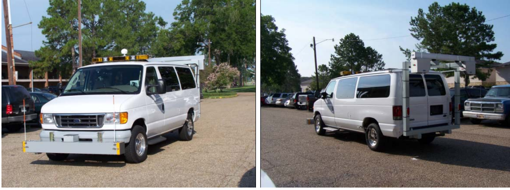
Figure 4 LTRC multi-functional digital highway data vehicle
