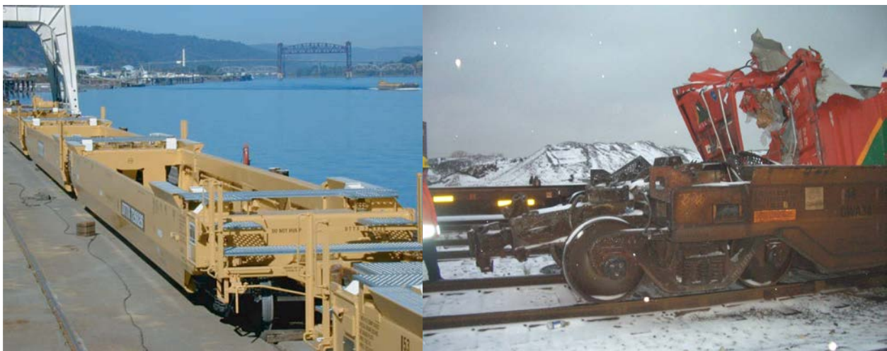
Figure A-2. Undamaged freight car (left) [14] and freight car involved in the accident (right).
