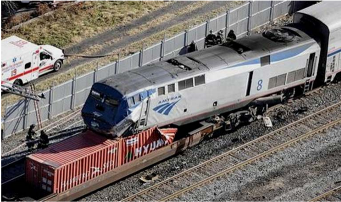
Figure A-14. The locomotive came to a stop on top of the freight car [4].
