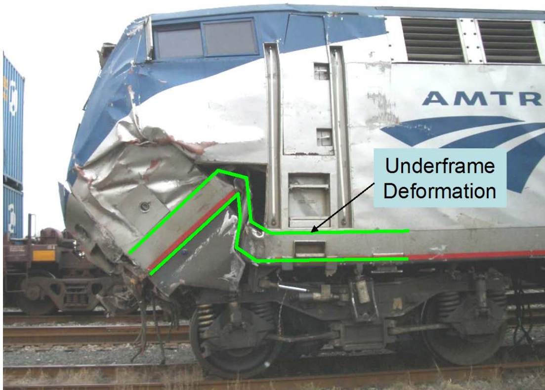
Figure A-9. Locomotive nose and underframe deformed inward and upward.
