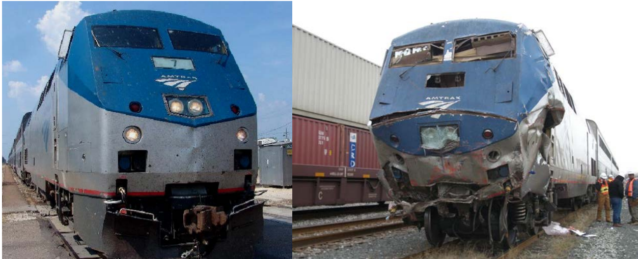
Figure A-1. Undamaged locomotive (left) [13] and locomotive involved in the accident (right).
