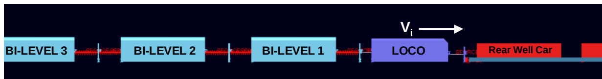
Figure A-27. Schematic of one-dimensional lumped-mass collision dynamics model of Chicago accident.
