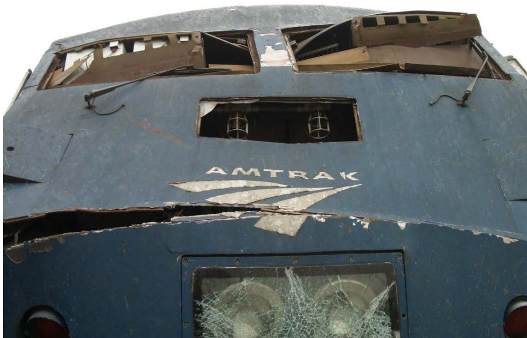
Figure A-10. Desktop components pushed through windows of locomotive cab.
