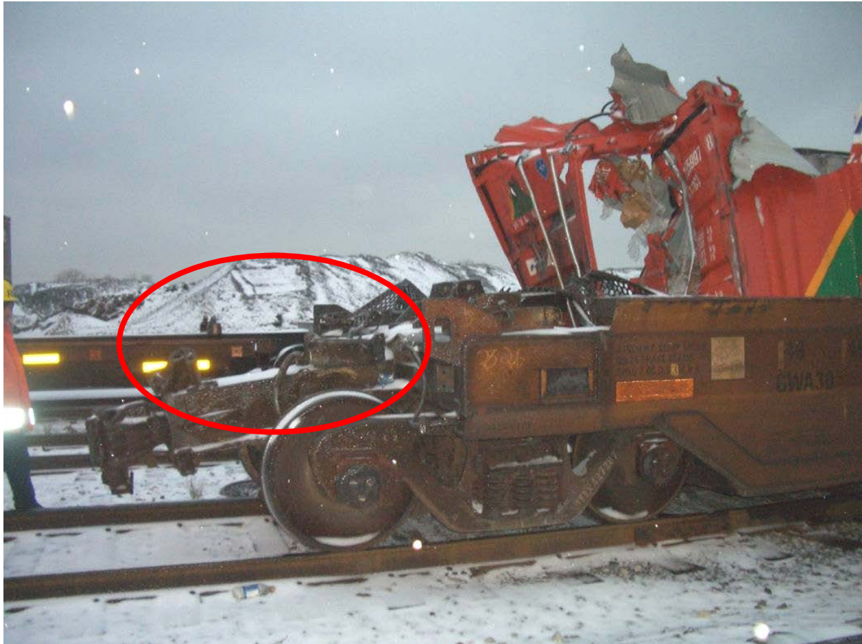
Figure A-8. Deformed draft sill of freight car.
