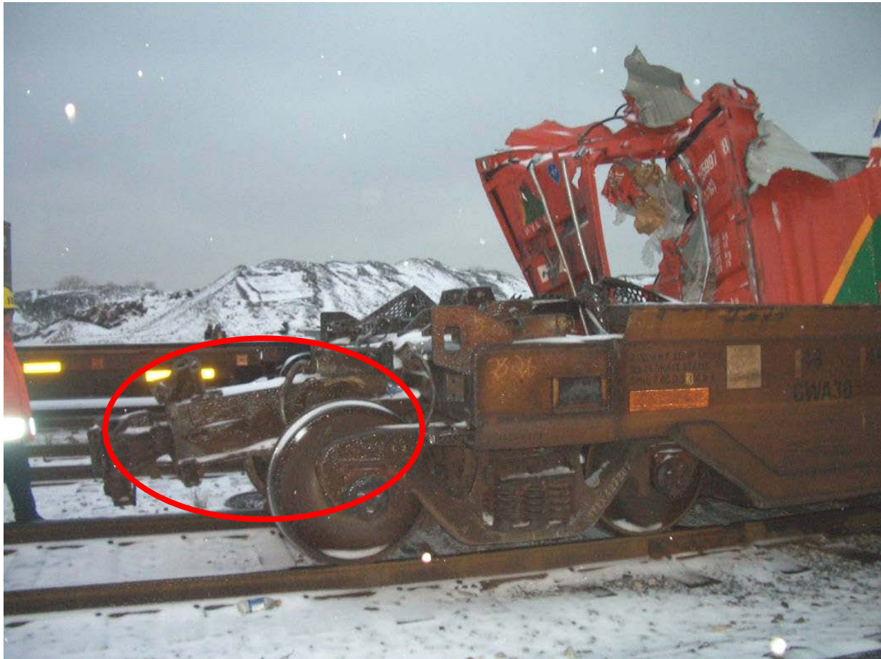
Figure 7. Deformed draft sill of freight car.
