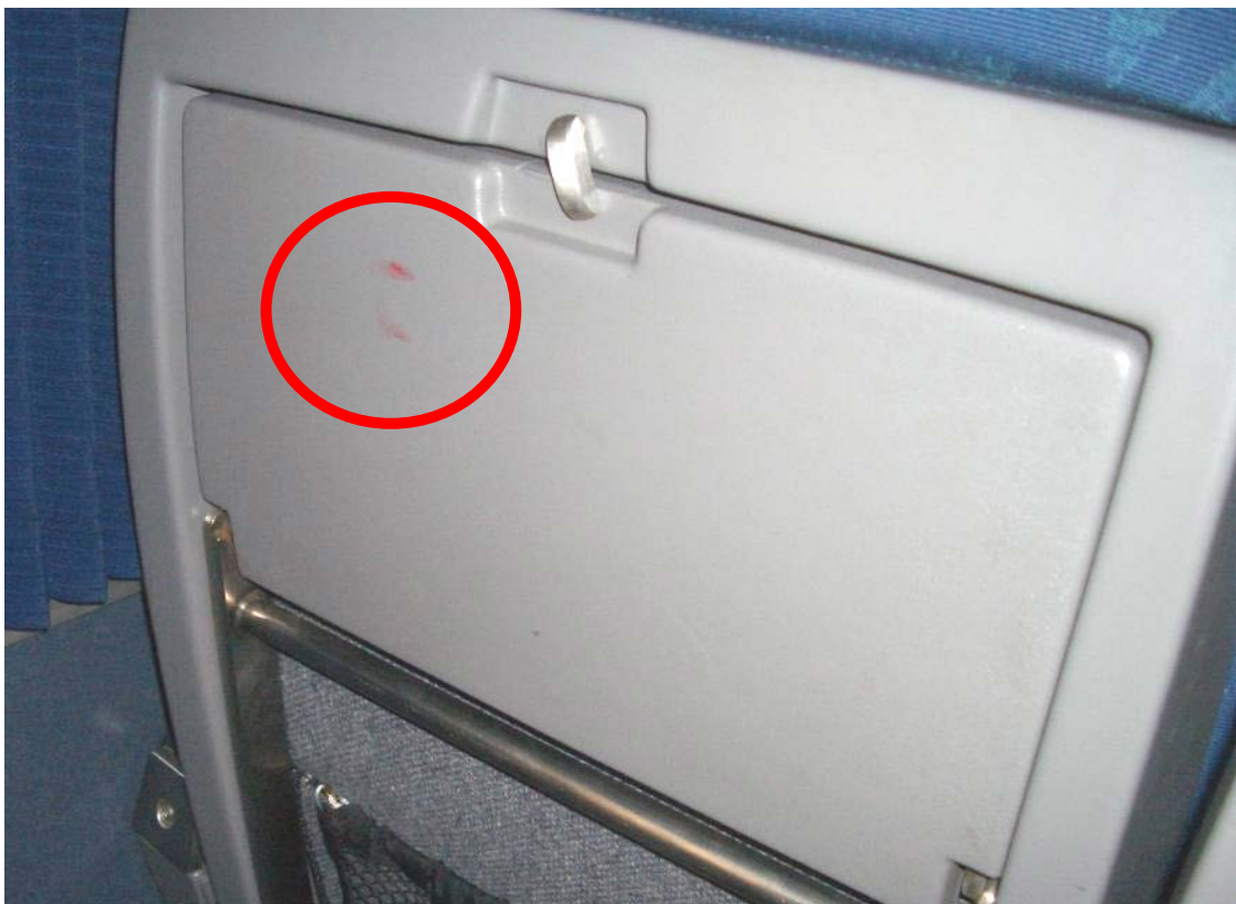
Figure A-25. Evidence of passenger injuries from impact with seat backs.
