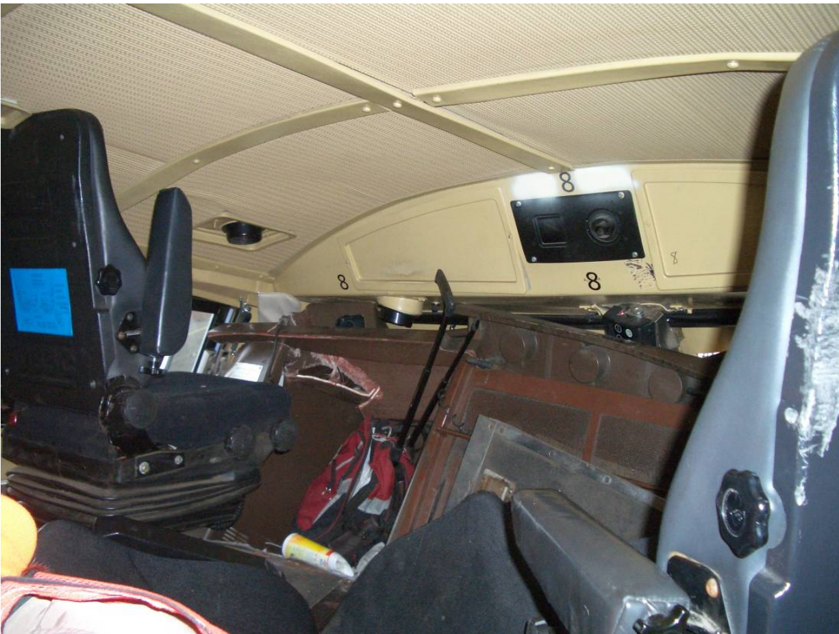
Figure 9. Locomotive interior cab damage and raised floor from impact.
