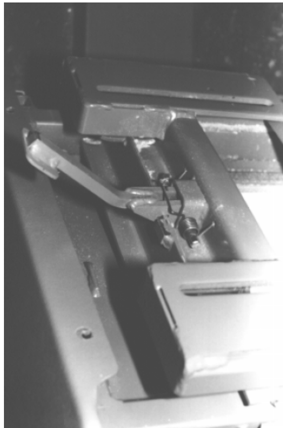
Figure A-33. Locking mechanism photograph, mechanism in the locked position.
