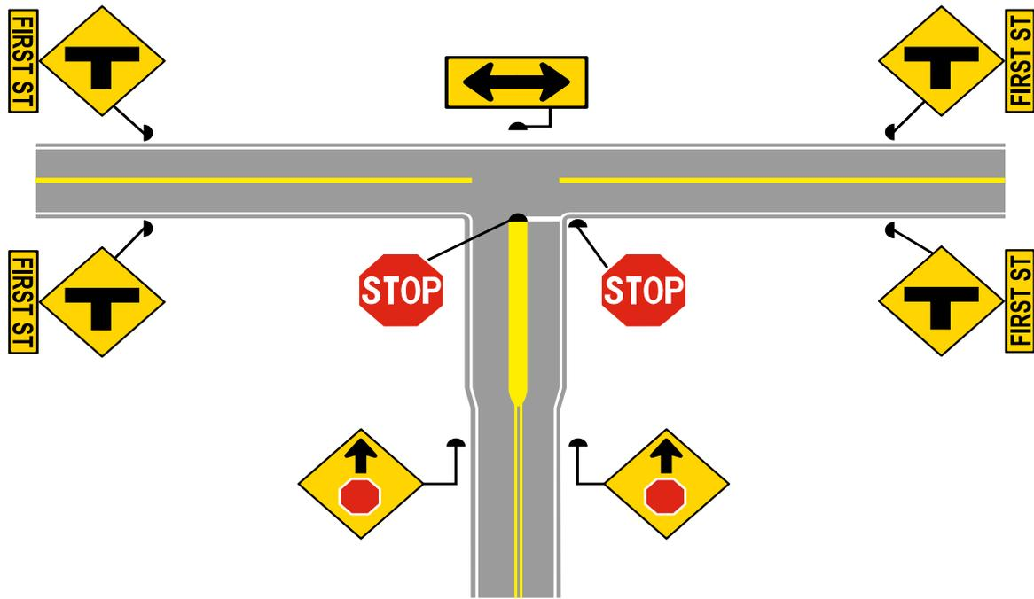
Figure 1: Traditional Sign Enhancements for Stop-Controlled Intersections
