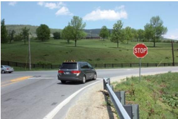
**Figure 3:** Stop Approach Activated LED Red Flashers on Perimeter of Stop Sign
