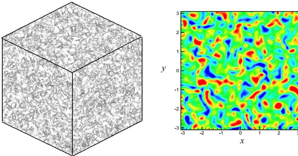
Figure 6. Plots illustrating the homogeneous turbulence flow field used for computing effect of turbulence on algae growth rate: (a)  $\lambda_2 = 0$  iso-surface in a three-dimensional perspective view, illustrating the vortex structures in the turbulent flow field, (b) contours of  $\omega_z$  in the  $z = 0$  cross-sectional plane
