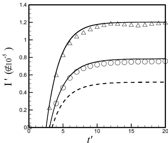
**Figure 7. Predicted dimensionless growth rate as a function of dimensionless time for cases with no flow (dashed line), predictions from the direct numerical simulation of Marshall and Haung (2010) for mixing with  $f_T = 0.36$  (circles) and  $f_T = 1.8$  (triangles), and the corresponding predictions from the stochastic Lagrangian model with the same turbulent kinetic energy and dissipation rate (solid lines).**
