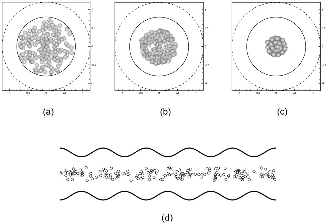
Figure 3. Time series showing particles focusing at the center of a corrugated tube for a case with Reynolds number  $Re = 10$ , from an end view. The dashed circle denotes the maximum (crest) of the tube corrugations and the solid circle represents the minimum (trough) of the corrugations. The side view in frame (c) is shown in frame (d).
