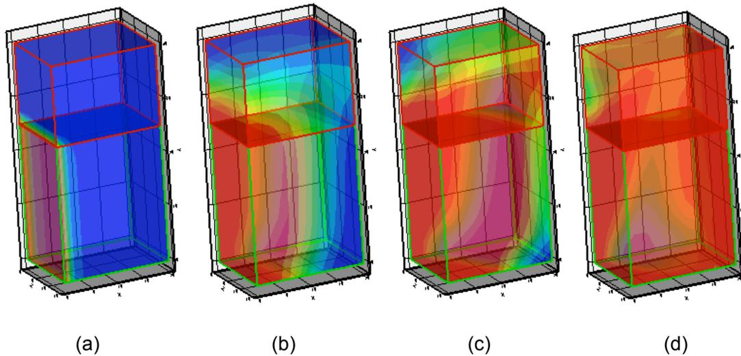
**Figure 1. Time series of three-dimensional temperature profiles in a rectangular combustor obtained from simulation of biofuel particles injected at the left-hand wall of the combustor. (Courtesy of Albert Ratner, University of Iowa.)**
