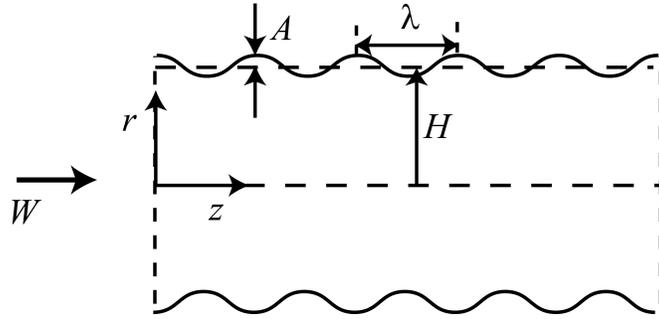
Figure 2. Schematic diagram of flow in a corrugated pipe.
