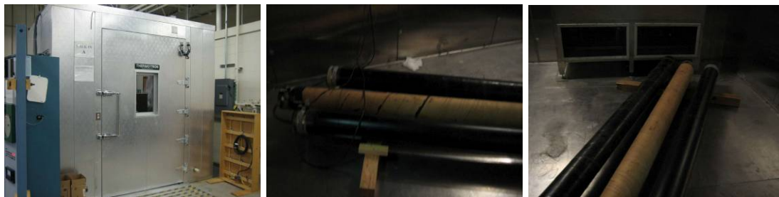
Figure 55. Environmental chamber (left) and three coated pipe samples (middle and right)
