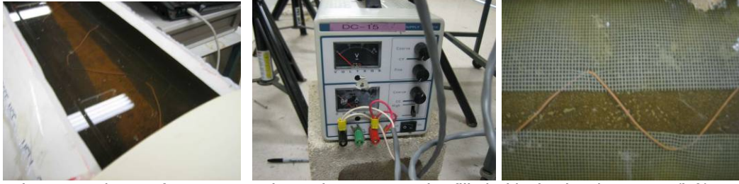
Figure 57. Photos of present experimental setup; PVC pipe filled with simulated seawater (left), power supply used to impress the electric current (middle), and fiberglass mesh wrapped around pipe sample (right)
