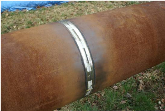
Figure 1. Alloy strips bonded to pipe with epoxy
