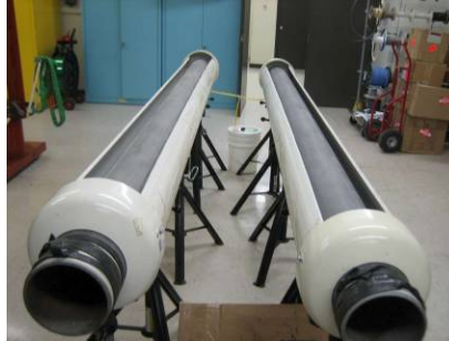
Figure 3. Experimental setup for investigation of corrosion effects on guided-wave attenuation.
