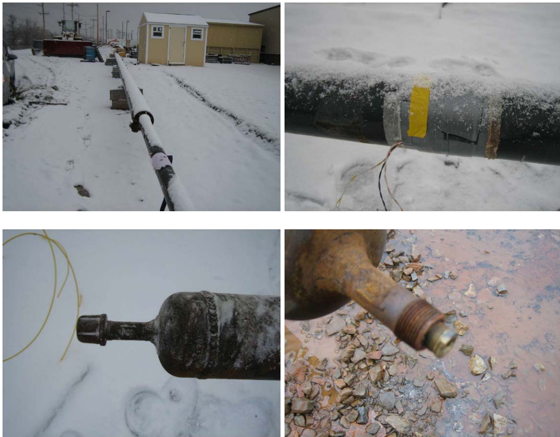
Figure 41. Photos taken during the testing on the 2 nd mockup: test pipe (top left), MsS probes (top right), and ends of test pipe (bottom)
