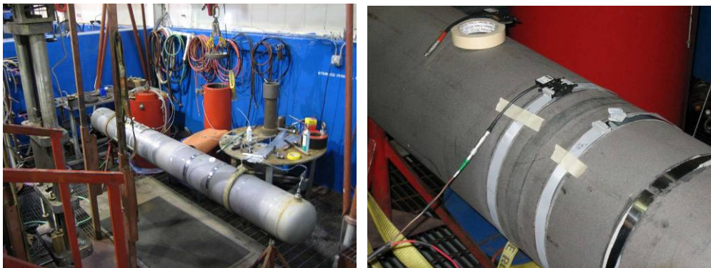
Figure 32. Photo of the 12-inch-OD pressure test sample (left) and the strips and MsS coils installed on the test sample (right)
