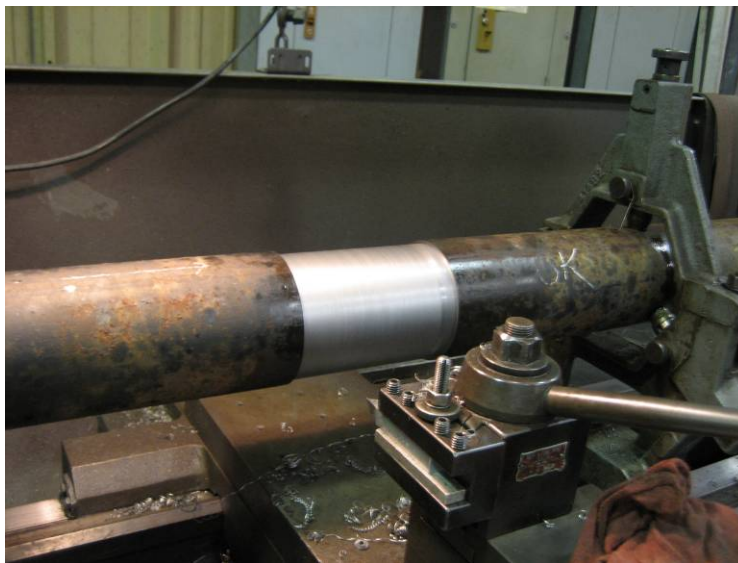
Figure 6. Photo of 4.5-inch-OD, 0.337-inch-wall pipe sample with 6-inch-long machined-in 360-degree notch
