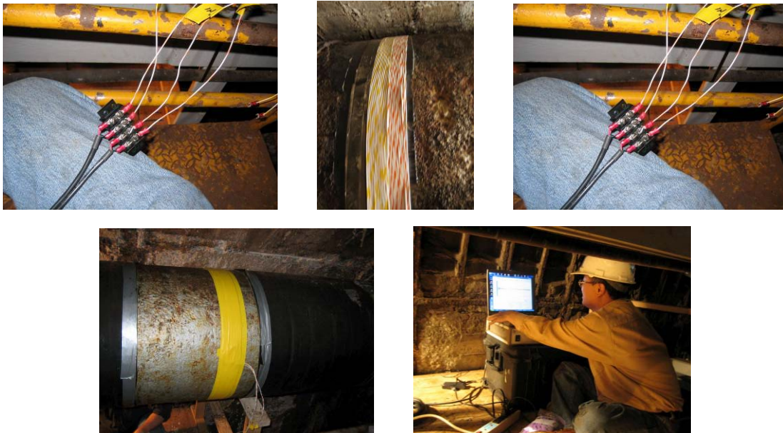
Figure 39. Photos of MsS testing on 26-inch OD gas pipeline: (a) a spool of #22 gauge insulated wire, (b) wires wound over the iron cobalt strips, (c) electrical connections to MsS instrument, (d) protective tape wound over the coils, and (e) acquisition of baseline data
