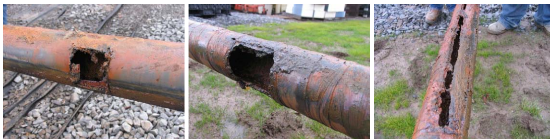
Figure 43. Photos of defects induced in the 1 st RG&E test pipe: large defects (left two) and 2.8% CSA defect around the weld location (right)
