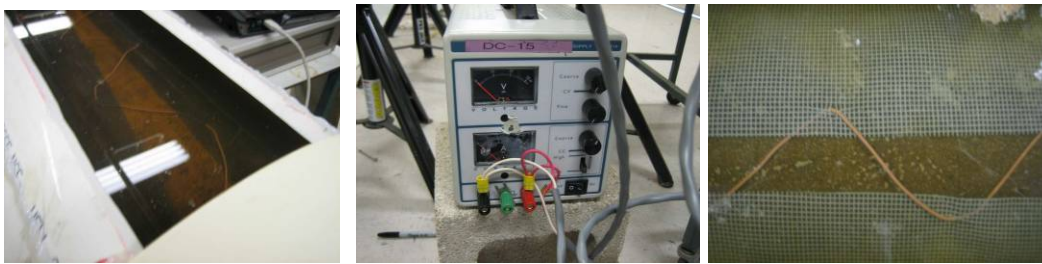
Figure 4. PVC pipe filled with salt water solution (left), power supply used to impress the electric current (middle), and fiberglass mesh wrapped around pipe sample (right)
