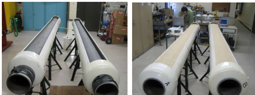
Figure 56. Photos of experimental setup for investigation of corrosion effects on guided-wave attenuation; samples placed in PVC pipes (left) and with the PVC pipe filled with sand (right)
