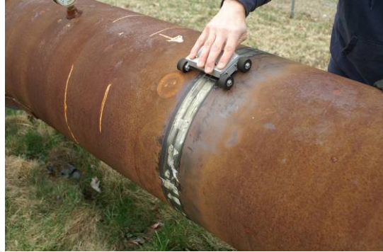
Figure 2. Manual magnetization of the alloy strips
