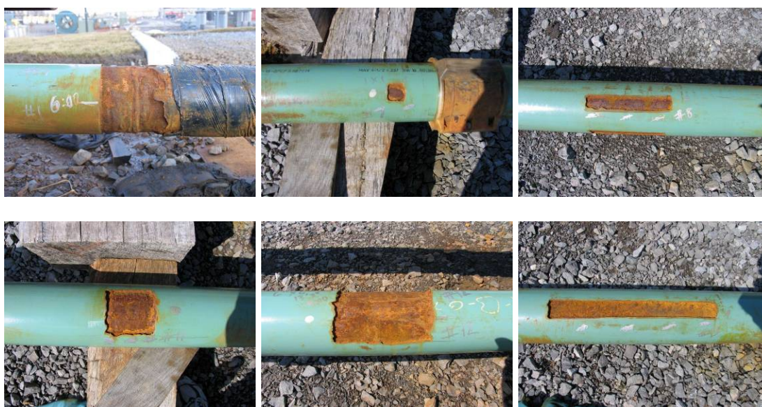
Figure 54. Photos of defects induced in the 2nd RG&E Test Pipe: RG&E defect ID Nos. 1, 7, 8 (top row from left to right) and 11, 12, 15 (bottom row from left to right)
