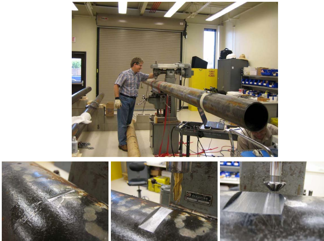
Figure 14. Photos of experimental setup and examples of notch defects of varying axial length and slope
