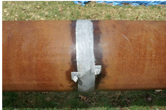
Figure 4. Wax coating applied over MsS assembly
