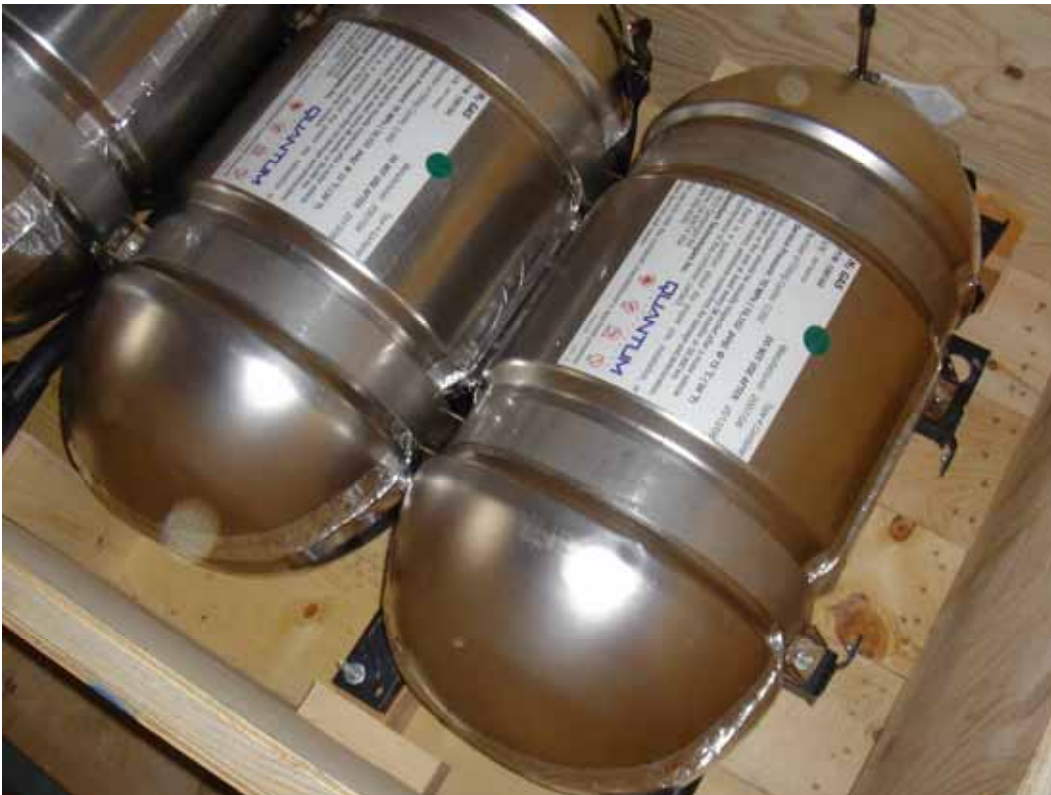
Figure 22 – Quantum fuel system assembly, complete with stainless steel shell covering.
