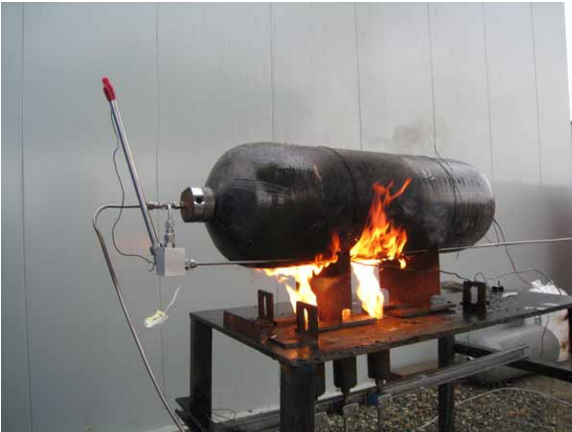
Figure 21 – Localized fire test of carbon fiber composite tank protected using a long SMA tube connected to a piston-activated PRD located outside of the fire.
