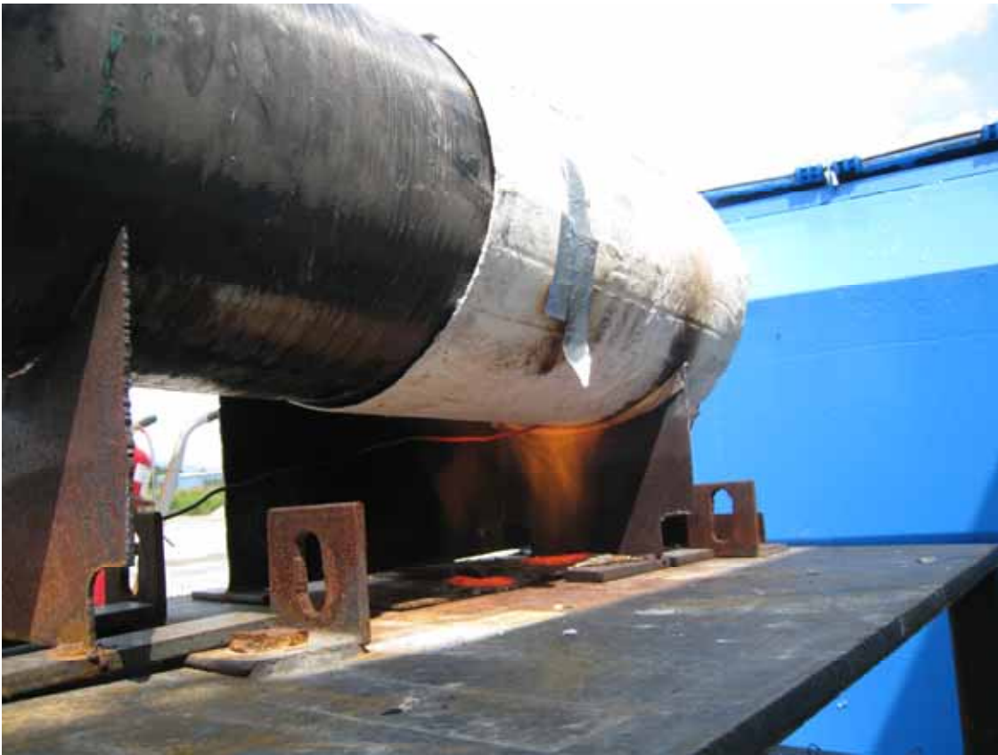
Figure 17 – Localized fire test of felt wrap after drying.
