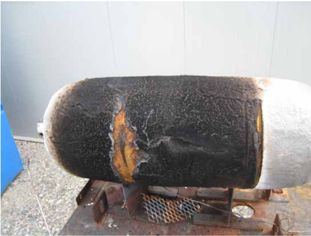
Figure 7 – Tank rotated after fire test to show foaming effect of coating. Note that the damaged area in the coating was caused by the metal support stand.
