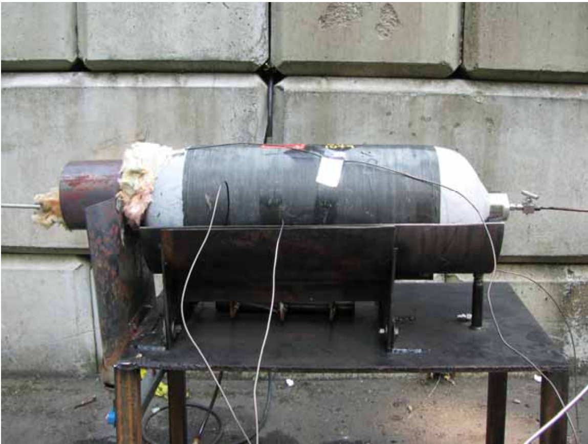
Figure 29 – Tank set-up for fire testing on the cradle.
