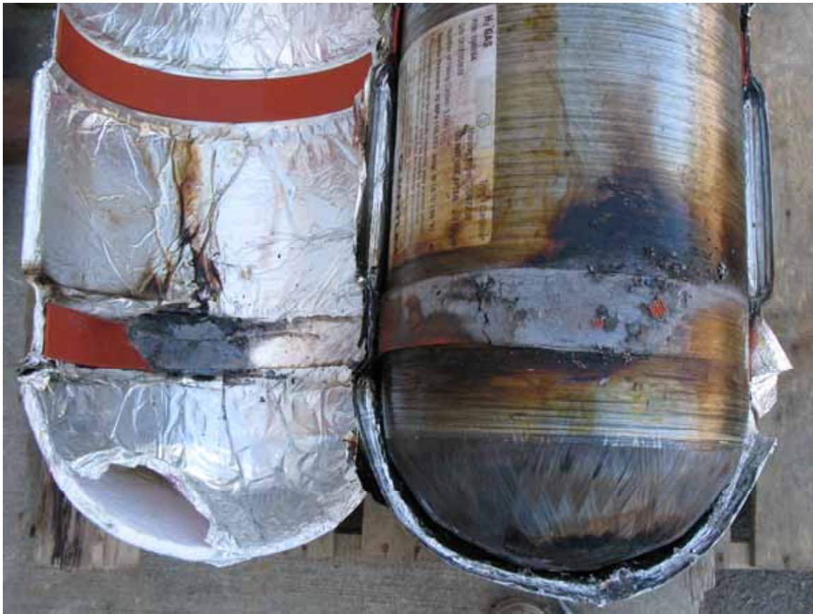
Figure 25 – Heat damage to surface of composite tank (right) revealed when heat-damaged half of shell folded open. Note the white ceramic blanket material exposed under the aluminum foil wrap (left).
