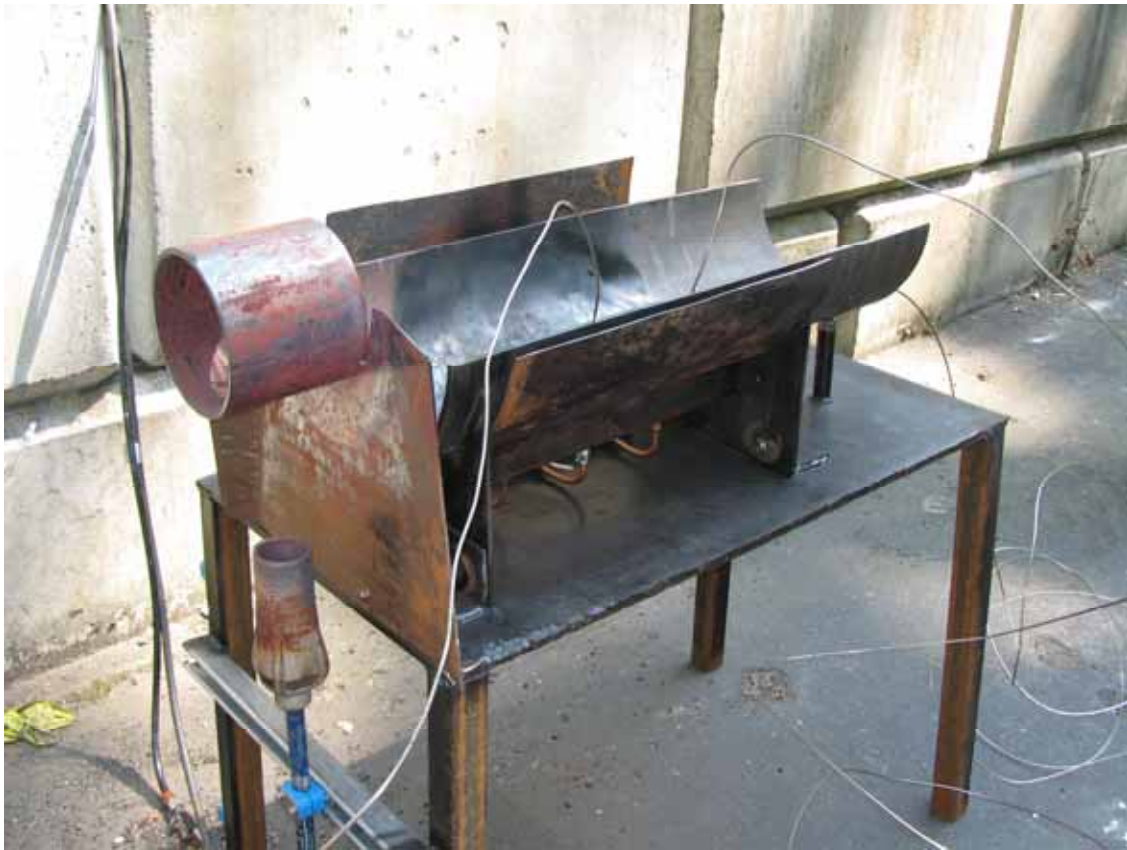
Figure 28 – Metal cradle used to generate different heat zones on a tank. In addition to burners located under the sidewall area, note the torch under the valve end.
