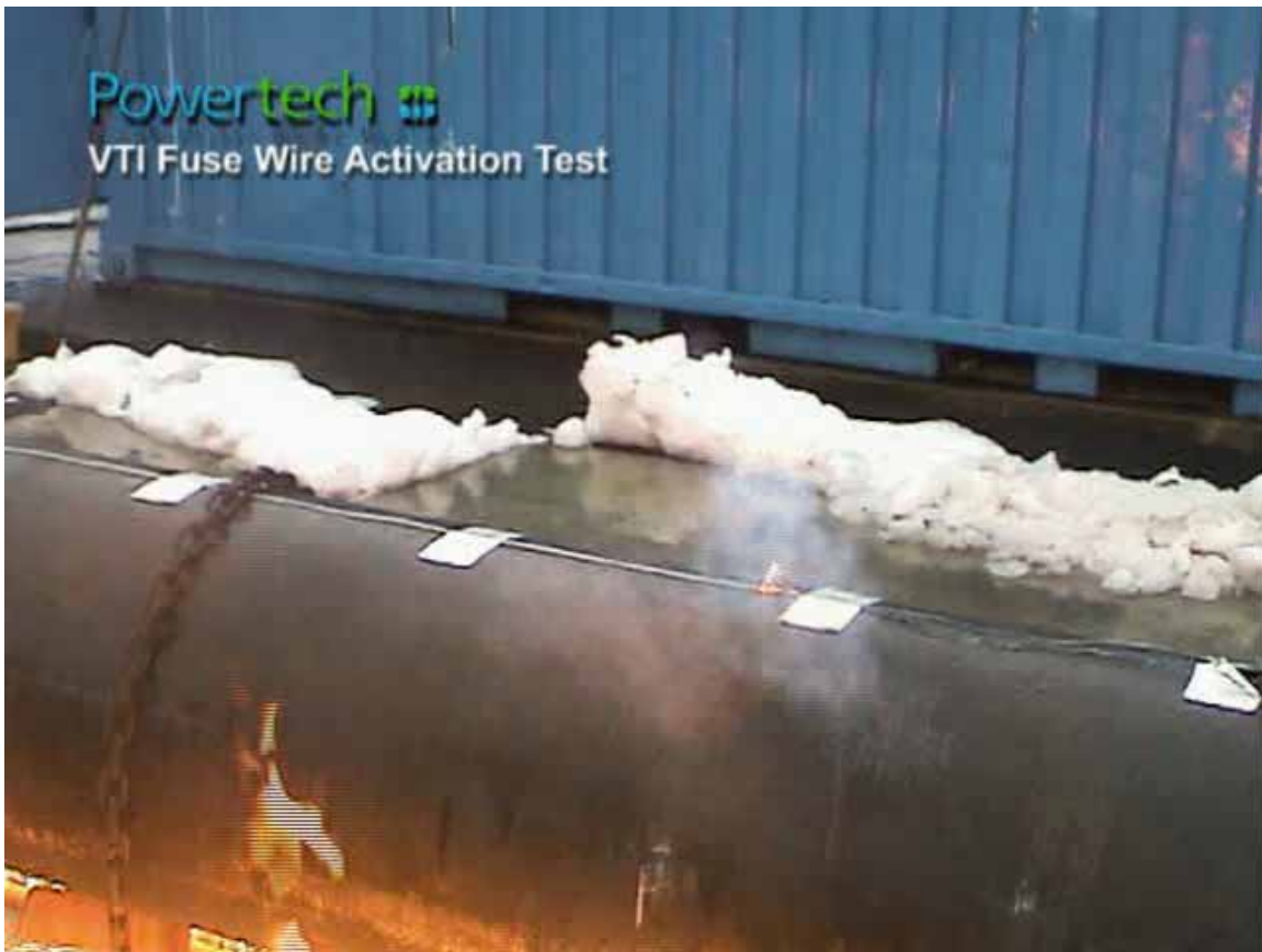
Figure 20 – Video capture from fire test of carbon fiber composite tank protected with fuse wire and TPRD at one end. Note the fuse wire burning along the top of the tank towards the TPRD (not visible in picture).
