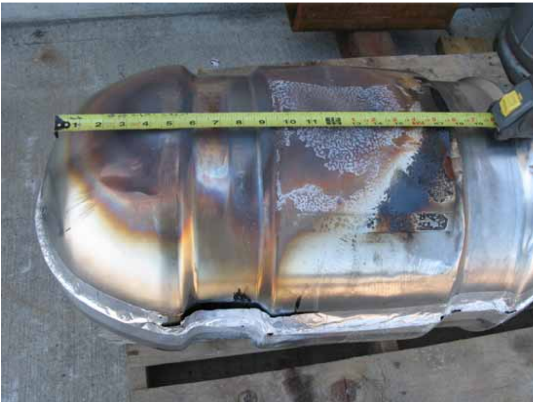
Figure 23 – Heat damage to stainless steel shell. Note that the length of the burn area is approximately 0.45 m.
