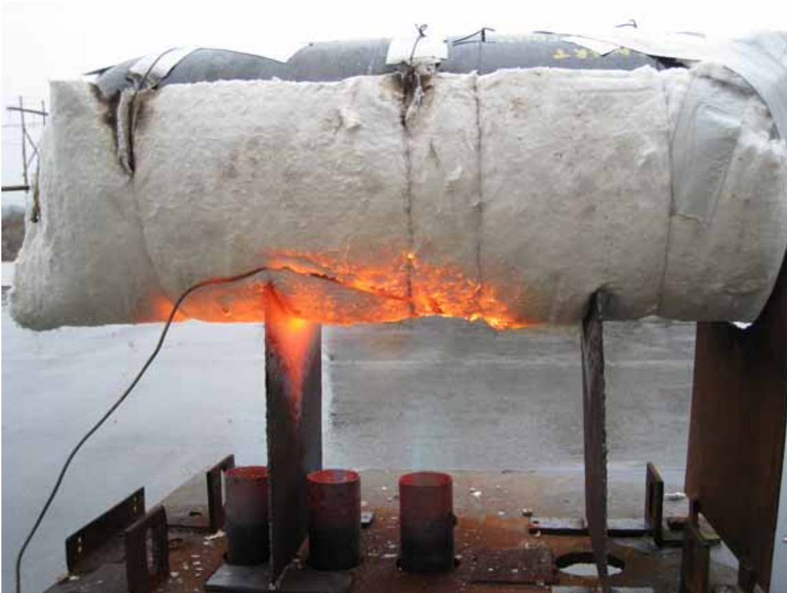
Figure 13 – Localized fire test of SuperWool 607 Plus blanket
