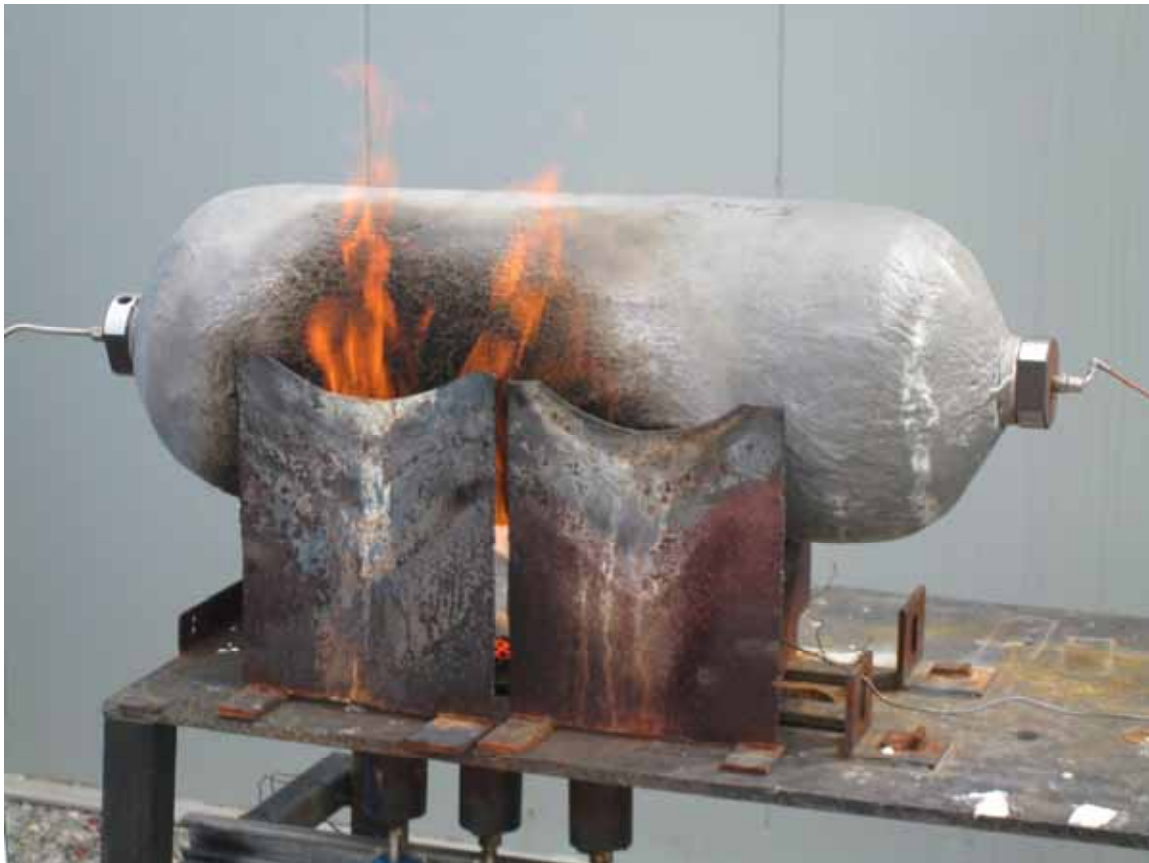
Figure 6 – Low pressure fire test of 5mm thick epoxy intumescent.
