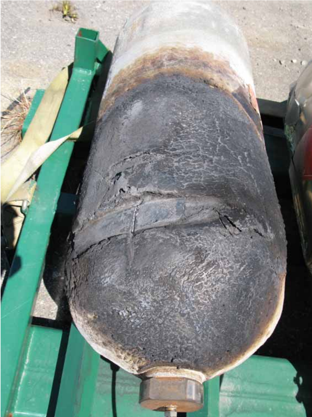
Figure 12 – Appearance of 8 mm thick epoxy intumescent coating after 30 minutes exposure to 900°C. Note that the flattened area is from handling after the test.
