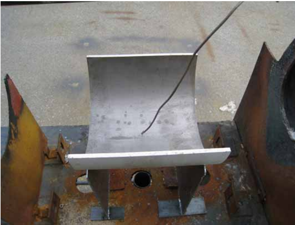
Figure 1 – Arrangement for fire testing steel pipe half-sections with one side coated by intumescent paint. Note thermocouple touching pipe surface on side opposite burner.
