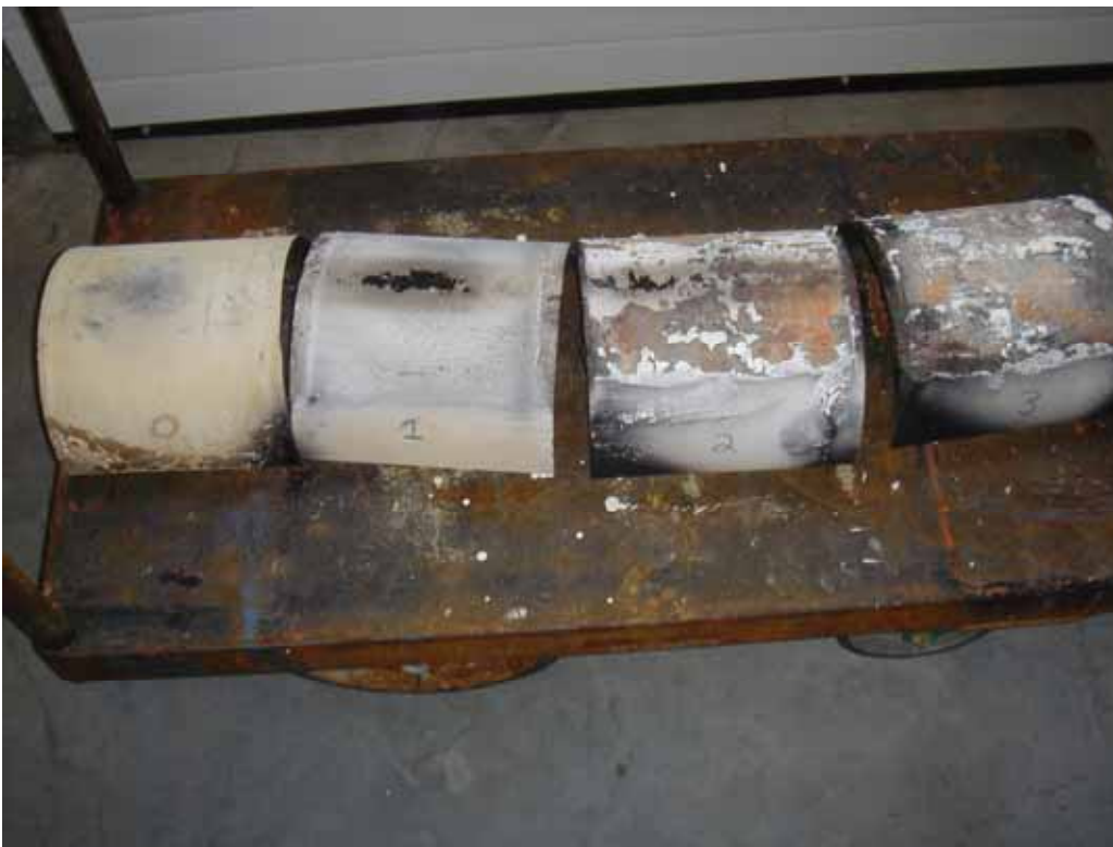
Figure 2 – Results of fire testing on PyroCide II paint coating of various thicknesses (#0 = bare steel, #3 = 3 coats of paint).
