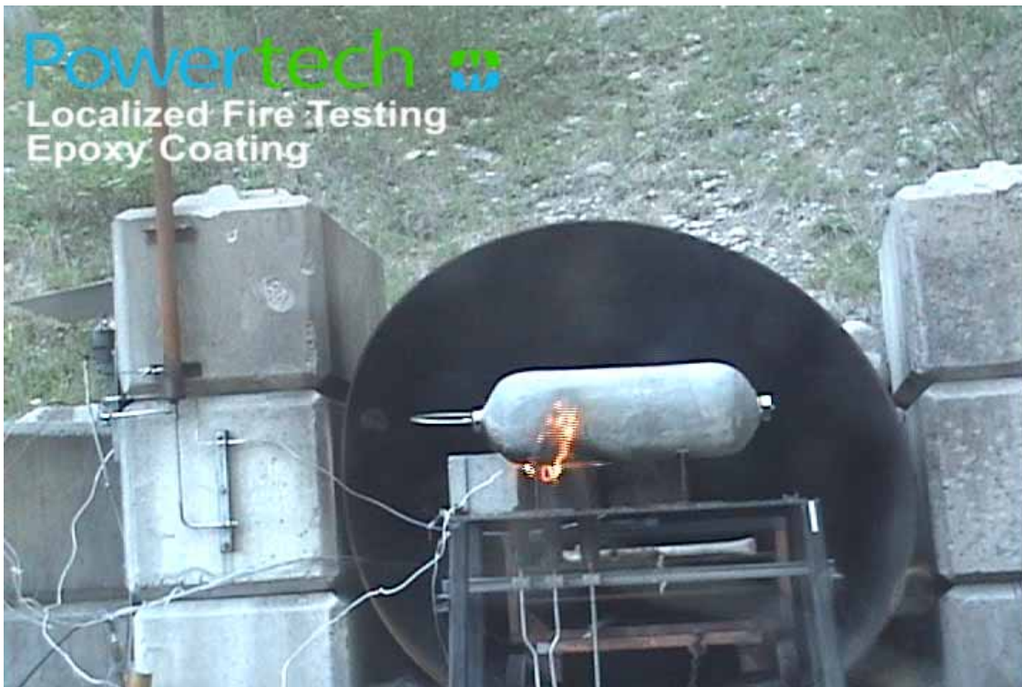
Figure 10 – Localized fire test of epoxy intumescent (8 mm thick) on carbon fiber tank containing 138 bar hydrogen for 30 minutes.
