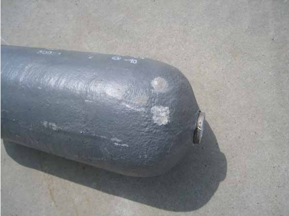
Figure 9 – Appearance of drop impact damage (rebound end) on dome end of 8 mm thick epoxy intumescent coating.
