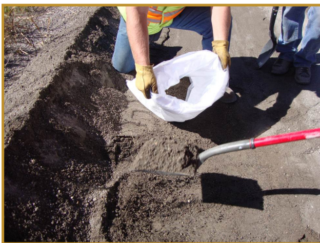
Figure 2 - Obtaining sample along the shoulder of I 90 near Bozeman Pass
