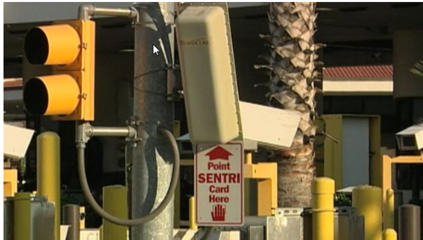
Figure 4. Photograph showing RFID card reader used in the SENTRI program (4).
