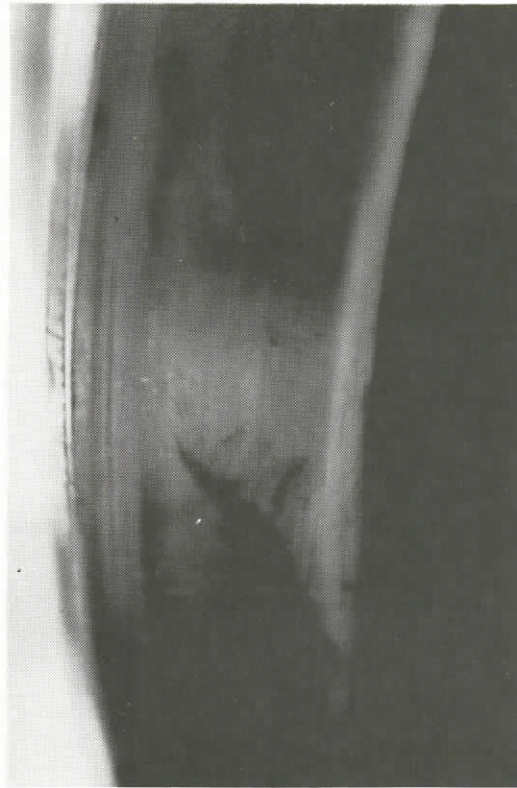
125. CLOSE-UP OF TREAD AND FLANGE DISCOLORATION
