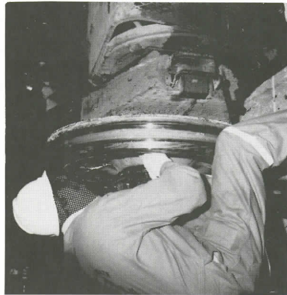
127. REMOVING WATERPROOF/PROTECTIVE COATING TO EXPOSE STRAIN GAGES ALSO SHOWING TRACTION MOTOR
