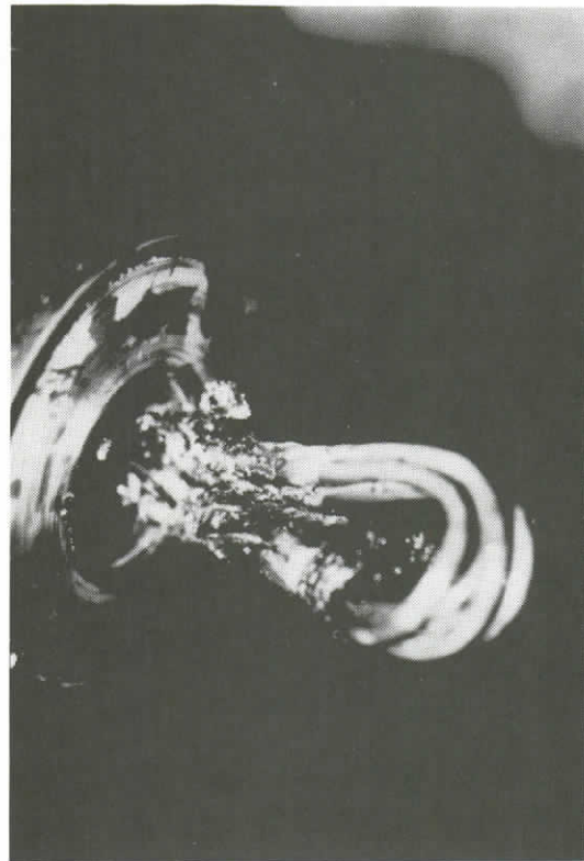
181. DETAIL OF DAMAGED WIRING PROTRUDING FROM AXLE BEARING BLOCK
