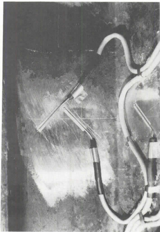
48. DETAIL OF STRAIN GAGES AS INSTALLED
