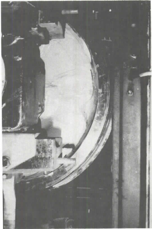
123. OVERHEATED WHEEL SHOWING PEALED PAINT AS RESULT OF THE HEAT
