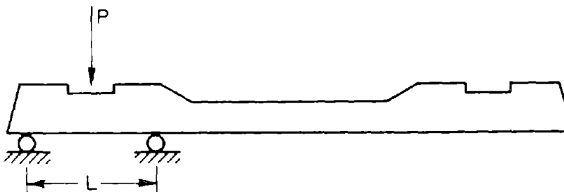
FIGURE 6-10c. LOADING CONFIGURATION TO GENERATE EI VALUE FOR RAIL SEAT SECTION Load Cell: L = 26 \text{ in.} RCCC Tie: L = 24 \text{ in.}
