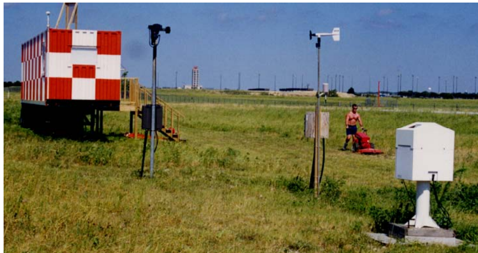
Figure 8. Meteorological Sensors: Present Weather (left), Wind/Temperature/Relative Humidity (middle), Ceiling (right)
