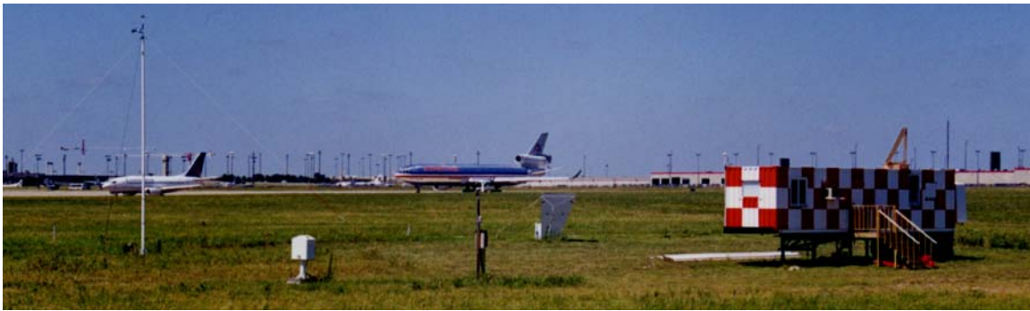
Figure 7. Additional Meteorological Sensors at Positive End of Windline
