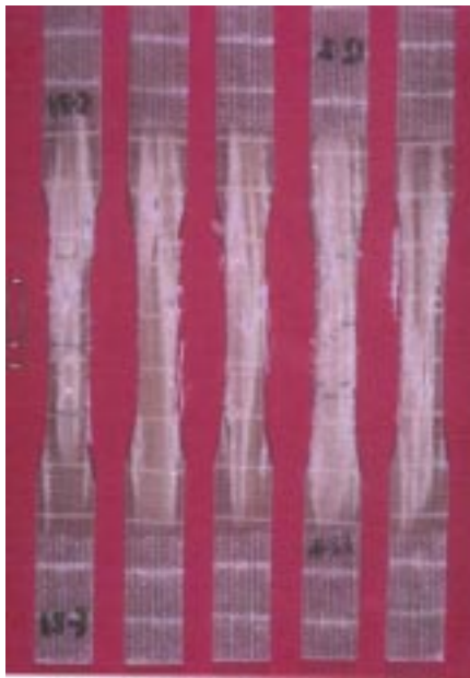
a. FRP laminate coupons after the tensile tests.
