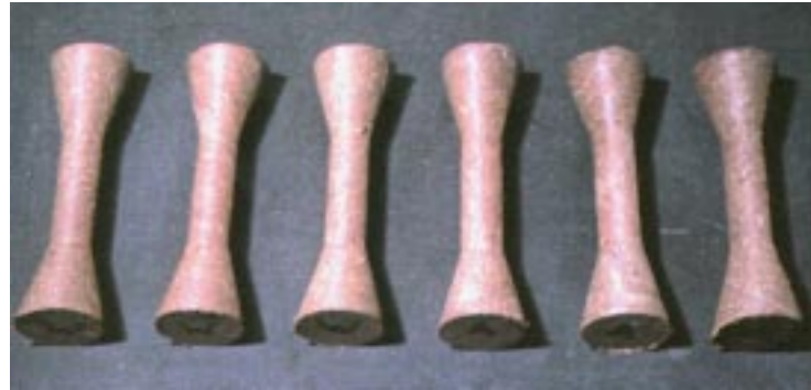
b. Some RPC tensile test specimens machined from the 152- × 203-mm (6- × 8-in.) beams.
