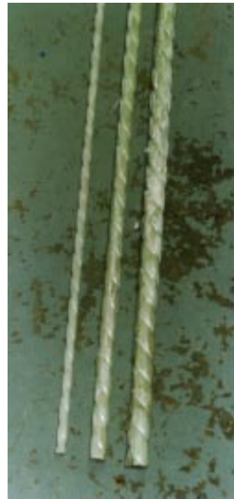
Figure 56. Examples of commercially available glass fiber reinforced composite rebars.
