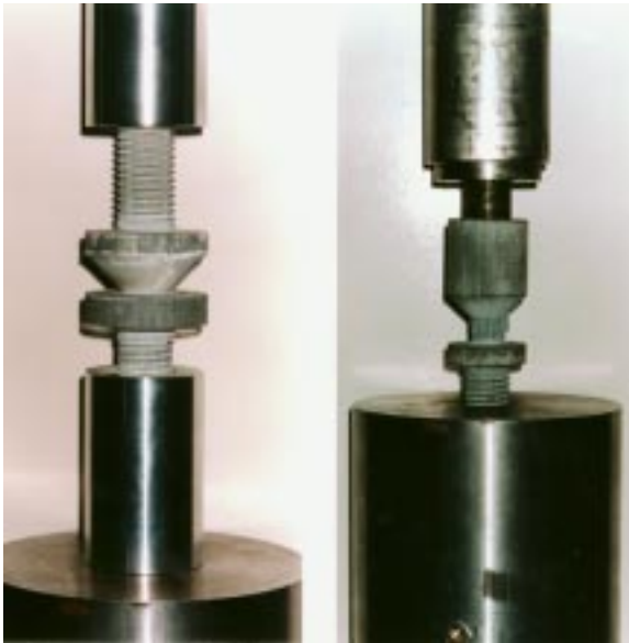
Figure 71. Tension testing of the male- (left) and female-threaded FRP breakaway coupler.
