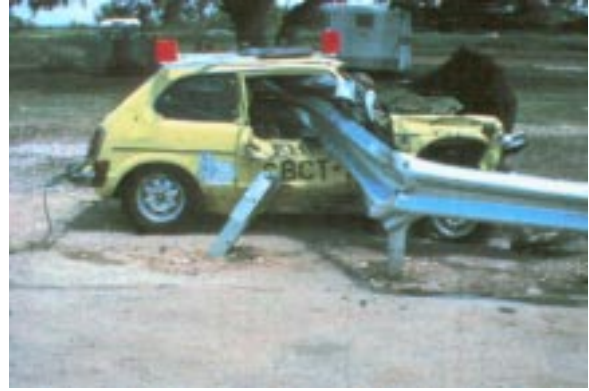
Figure 14. BCT speared on a 817.2-kg (1800-lb) car.
