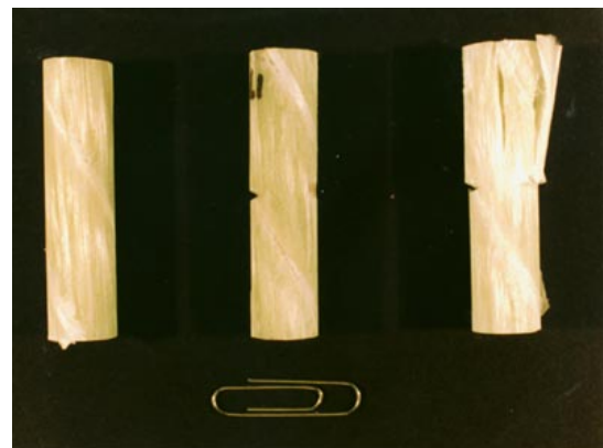
Figure 67. Unnotched, notched, and notch-impact-tested specimens.
