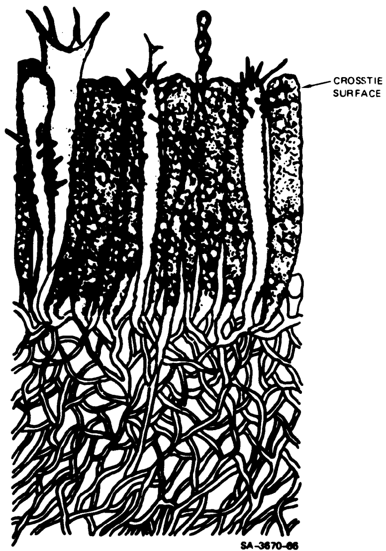
FIGURE 4.1 CROSS-SECTION VIEW OF DECAY FUNGI ATTACK
