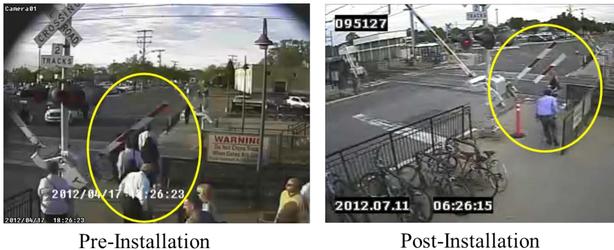
Figure 17. Examples of Descending Violations Pre- and Post-Installation
