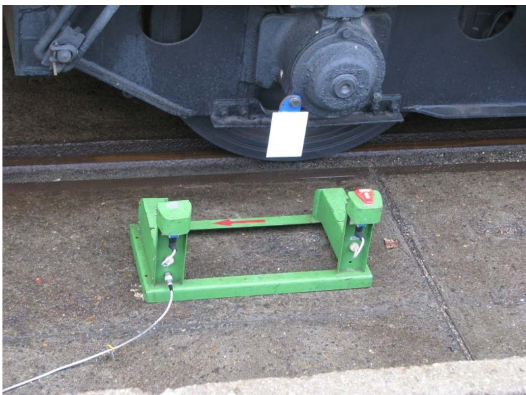
Figure 54. Stroke measurement with photo sensors
