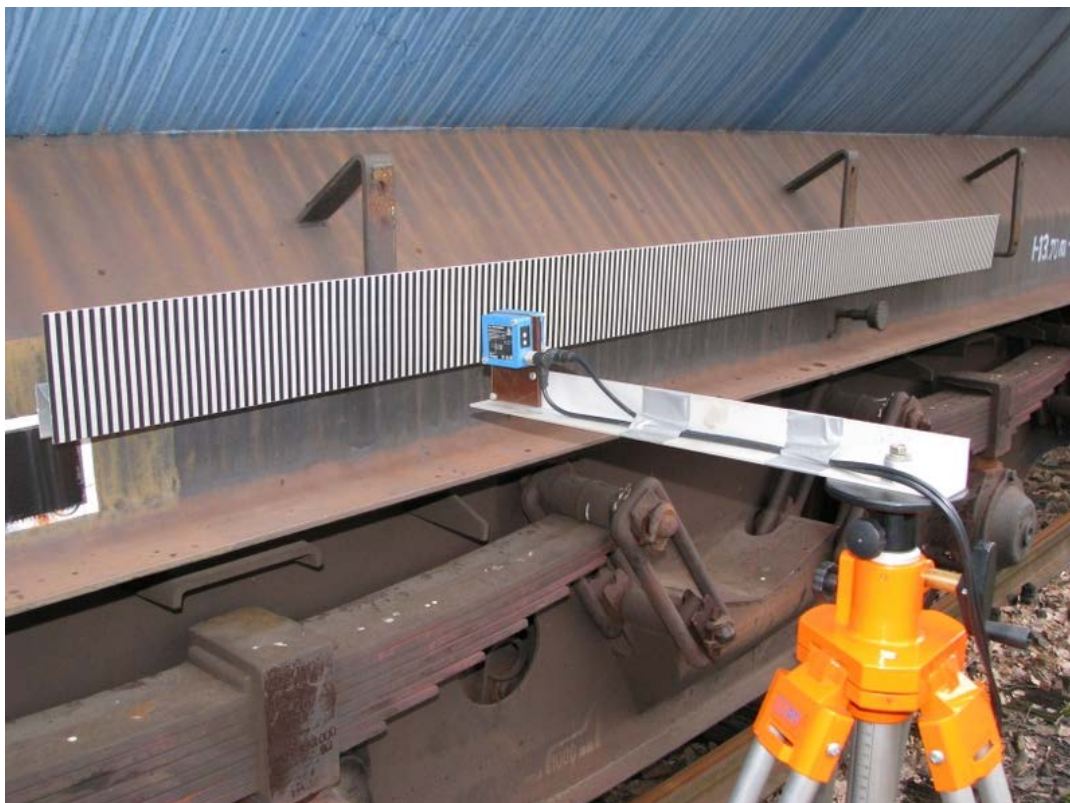
Figure 53. Stroke measurement with laser & ruled strip
