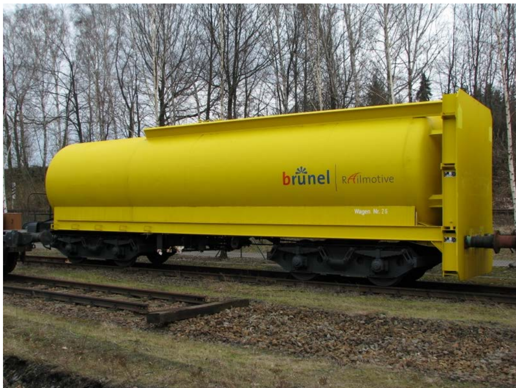
Figure 49. The 78-metric-ton impacting rail car
