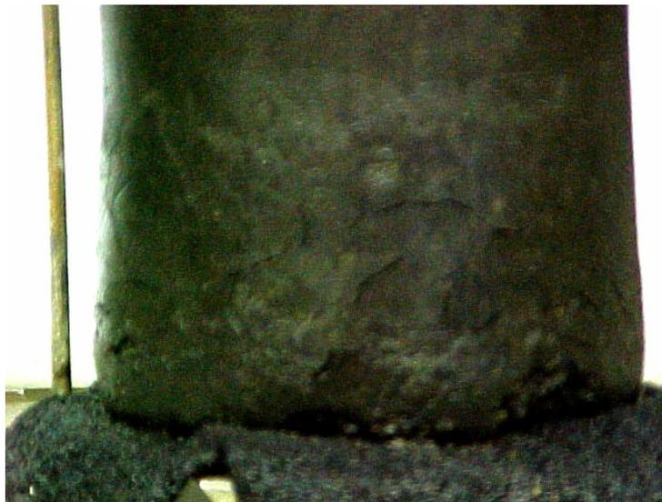
**Figure 72. SGS CFA after one freeze-thaw cycle**
