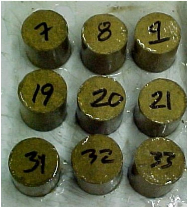
Figure 64. Paleosol and fly ash cured at 100° F after soaking
