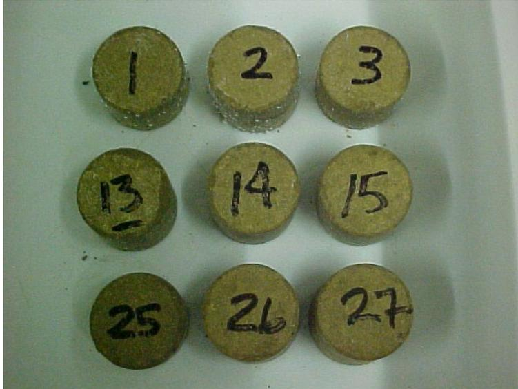
Figure 63. Paleosol and fly ash cured at 70° F after soaking
