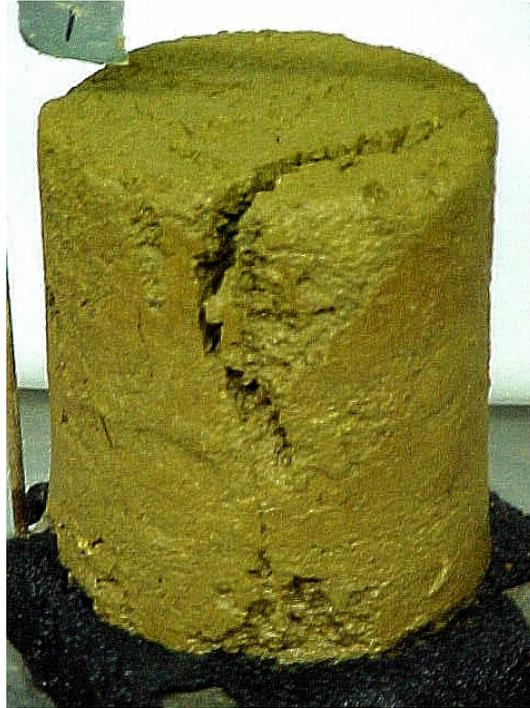
**Figure 75. Le Grand loess after the second freeze-thaw cycle**
