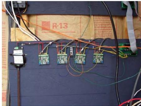
Soil strain data acquisition
