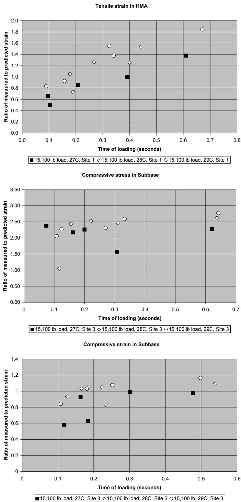
FIGURE 8 Comparison of predicted and measured responses
