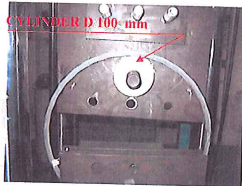
Figure 2. Upper part of the device devoted to the load application on a single ring.
