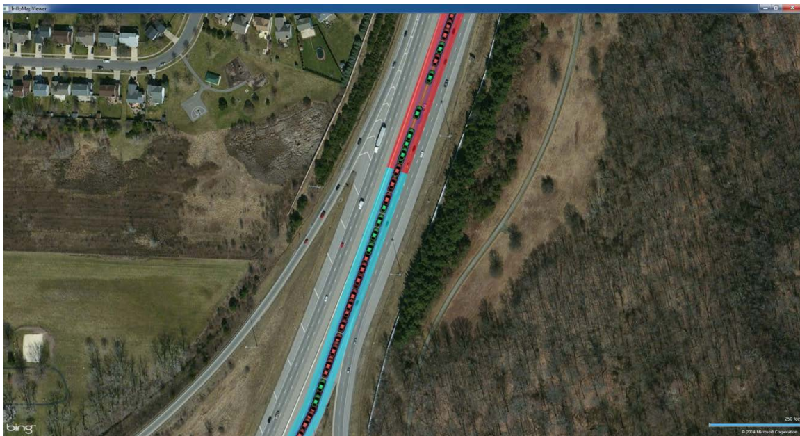
Figure 4-20. INFLO Database Map Viewer Displaying Vehicle BSM data with Queue Warning and Speed Harmonization Message Overlay on Satellite Image from Microsoft Bing ®. Traffic is flowing Northbound or upwards in the figure.
