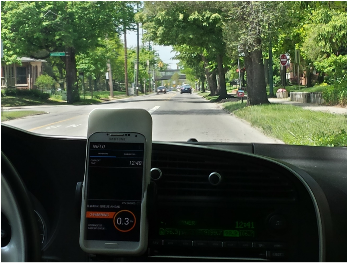
Figure 8-6. Queue Ahead Message Displayed Correctly on Battelle Connected Vehicle Test Loop
