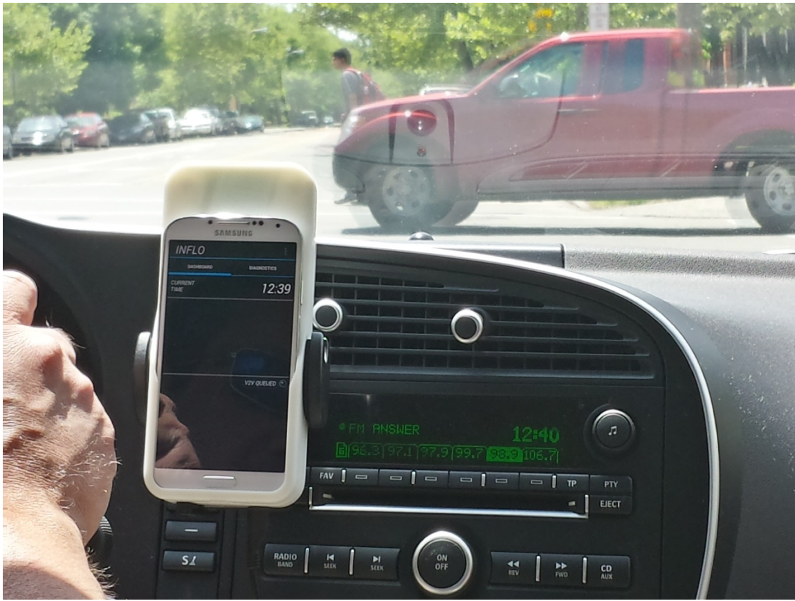
Figure 4-15. Nomadic Device Mounted in Vehicle showing Android Samsung 4 Cellular Phone in Arada Backpack DSRC Radio
