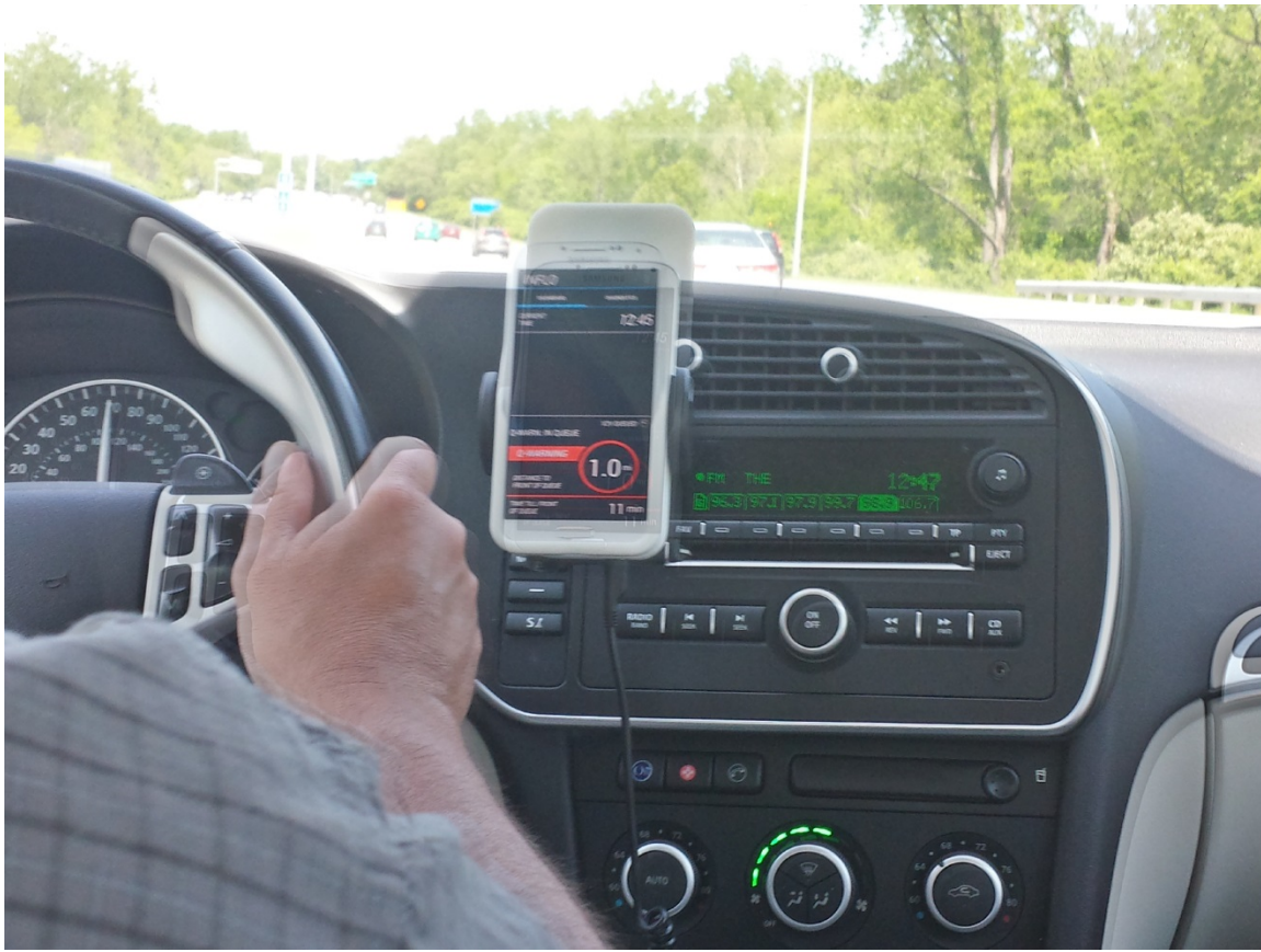
Figure 8-20. In-Queue Message While Traveling State Route 315 indicating Queue is 1 Mile in Length and Will Take 11 Minutes to Traverse
