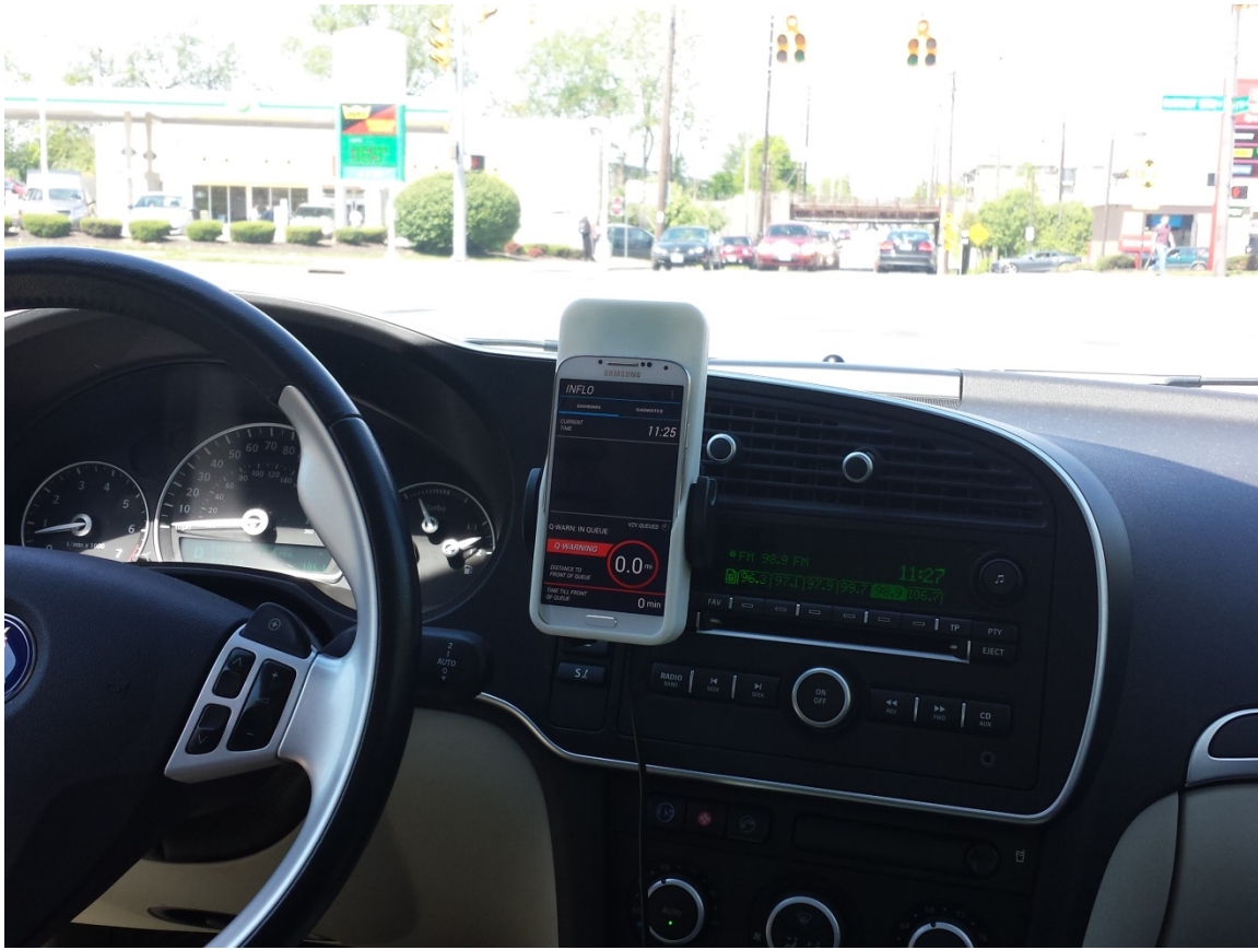
Figure 8-8. In-Queue Message Displayed Correctly on Battelle Connected Vehicle Test Loop
