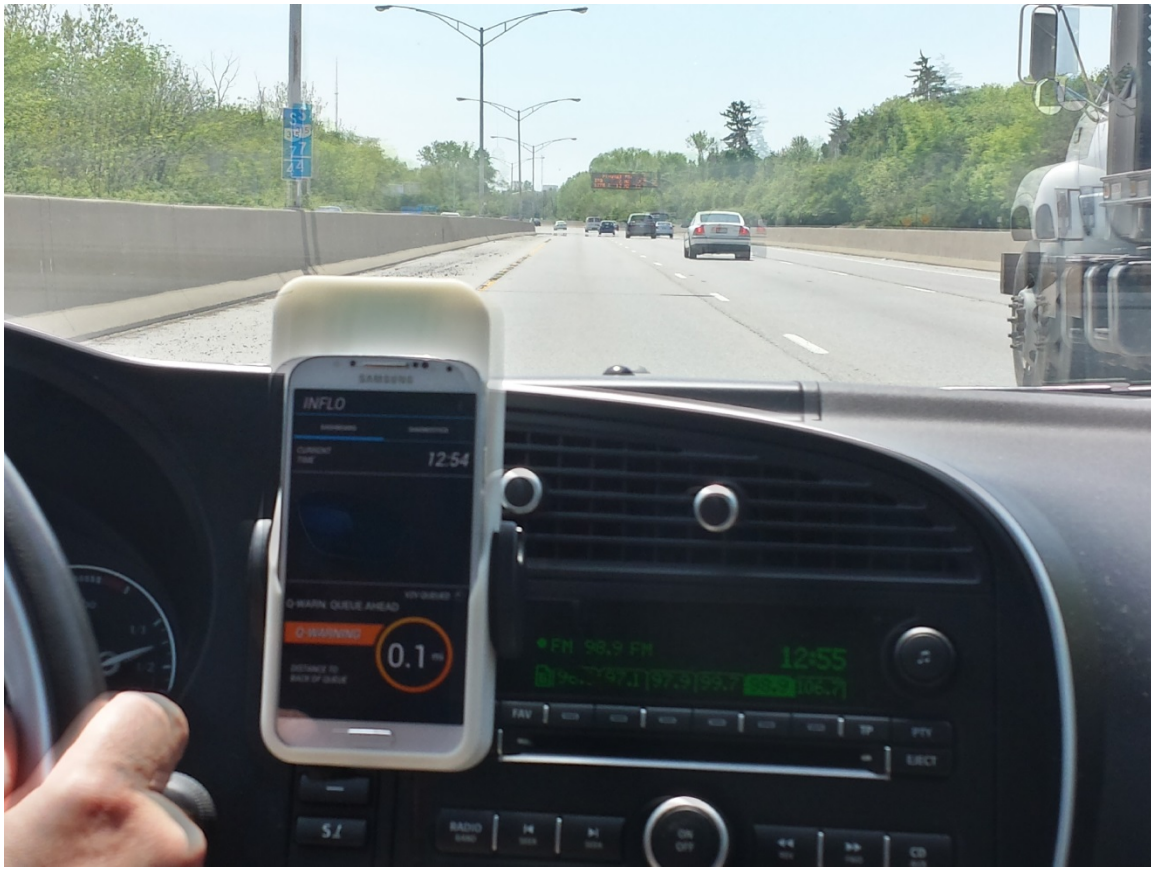
Figure 8-18. Queue Ahead Message While Traveling State Route 315 Indicating Back of Queue 0.1 mile Ahead
