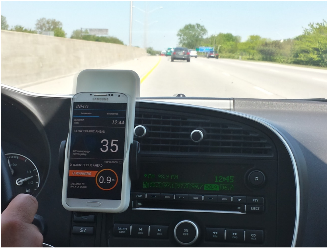
Figure 8-19. Queue Ahead and Speed Harmonization Recommended Speed Message While Traveling State Route 315
