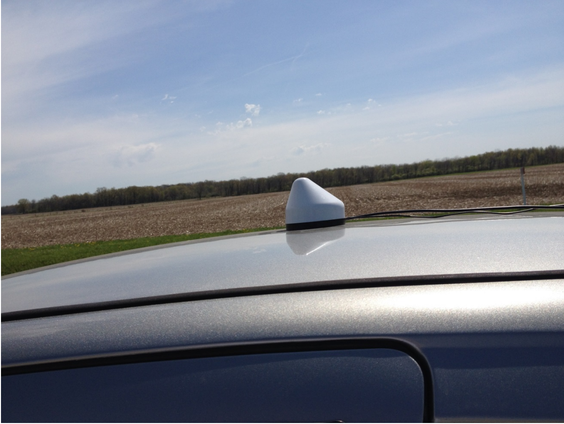
Figure 8-27. External DSRC and GPS Antenna Used for V2V DSRC Communications
