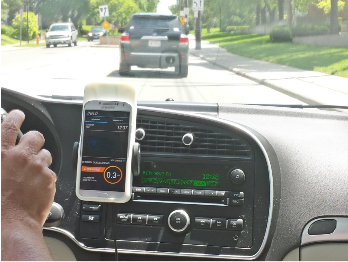
Figure 8-9. Queue Ahead Message Displayed Correctly on Battelle Connected Vehicle Test Loop
