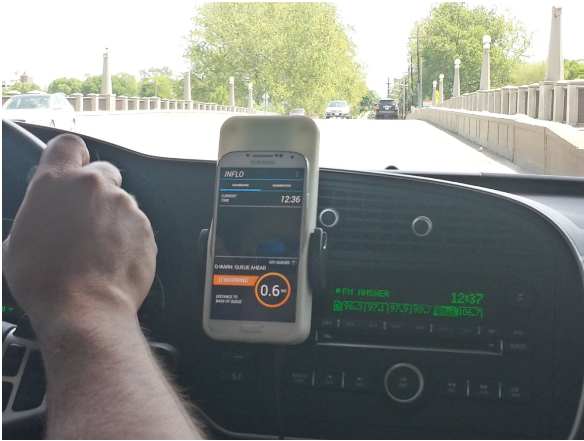
Figure 8-7. Queue Ahead Message Displayed Correctly on Battelle Connected Vehicle Test Loop
