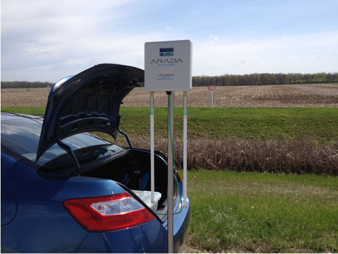
Figure 8-28. RSU to Demonstrate V2I Communications
