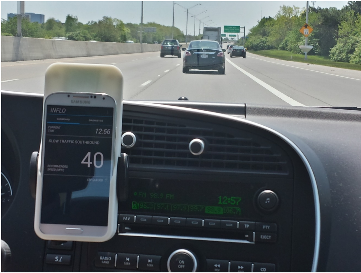
Figure 8-17. Speed Harmonization Message Display with Recommended Speed While Traveling on State Route 315
