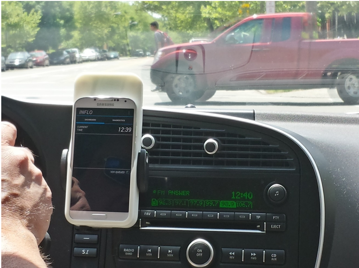
Figure 8-5. Nomadic Device Mounted in Vehicle showing Android Samsung 4 Cellular Phone in Arada BackPack DSRC Radio
