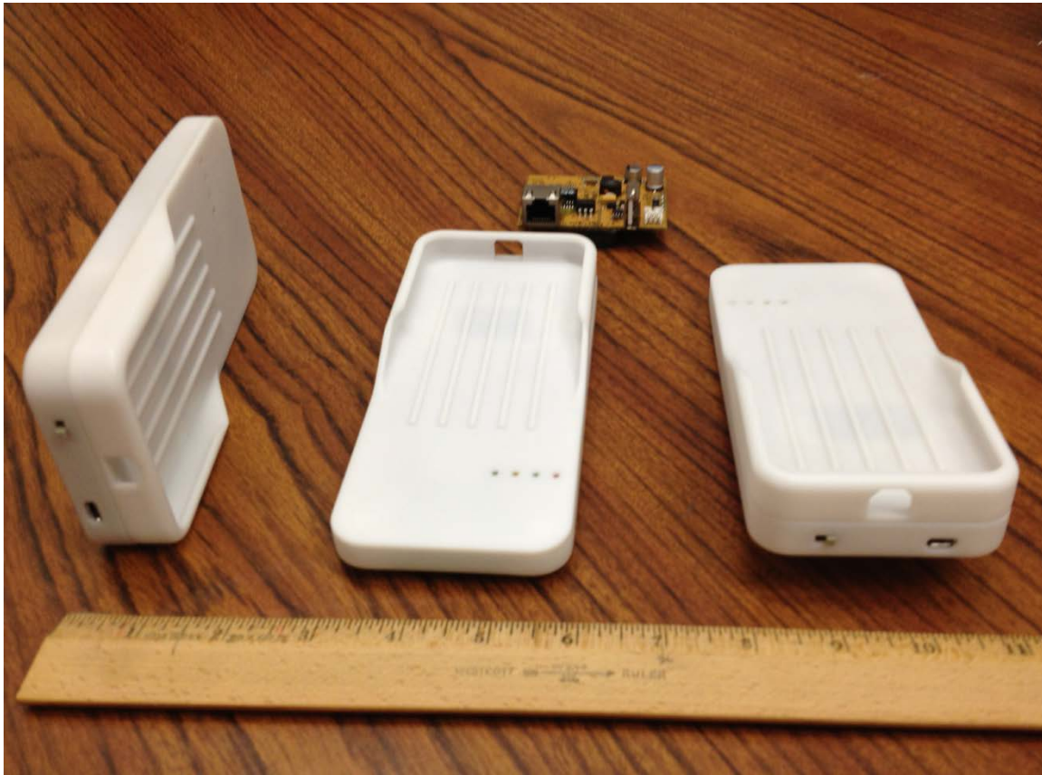
Figure 4-14. Nomadic Device DSRC Radio Module in the Backpack Form Factor for use with the ANDROID Mobile Device
